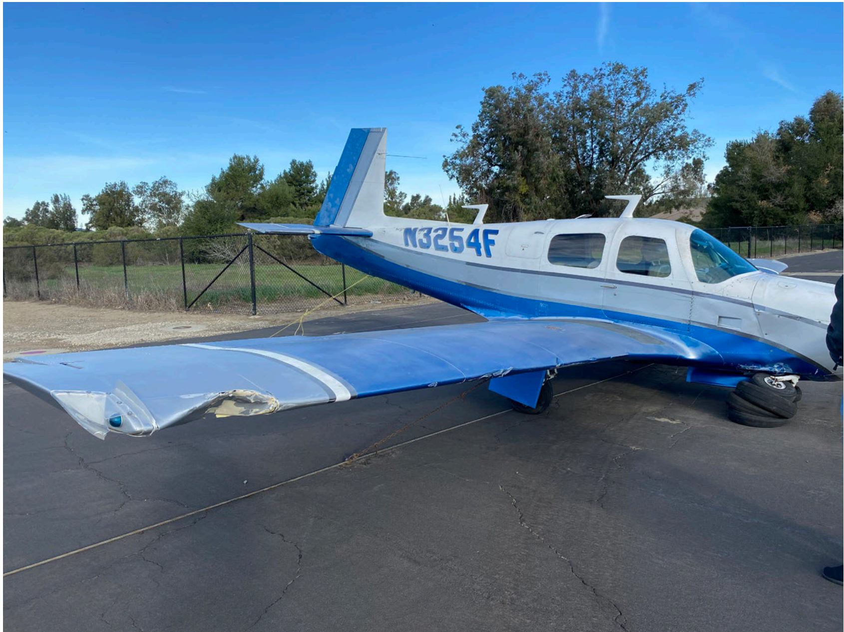
Photo 2 - Right Side of Airplane with damage to the wing tip and length of the wing. (Photo Courtesy of FAA)
