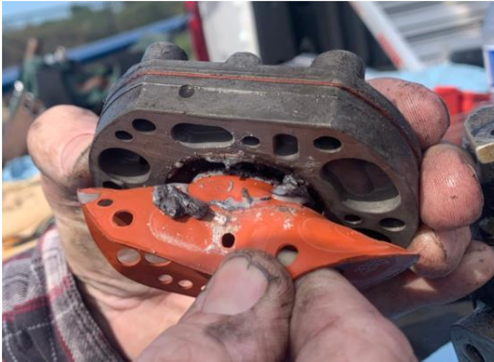
Grey sludge material found in the fuel flow diaphragms
