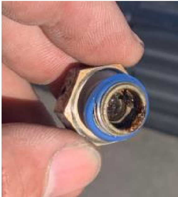
Fuel injection servo filter plug with rust and black material
