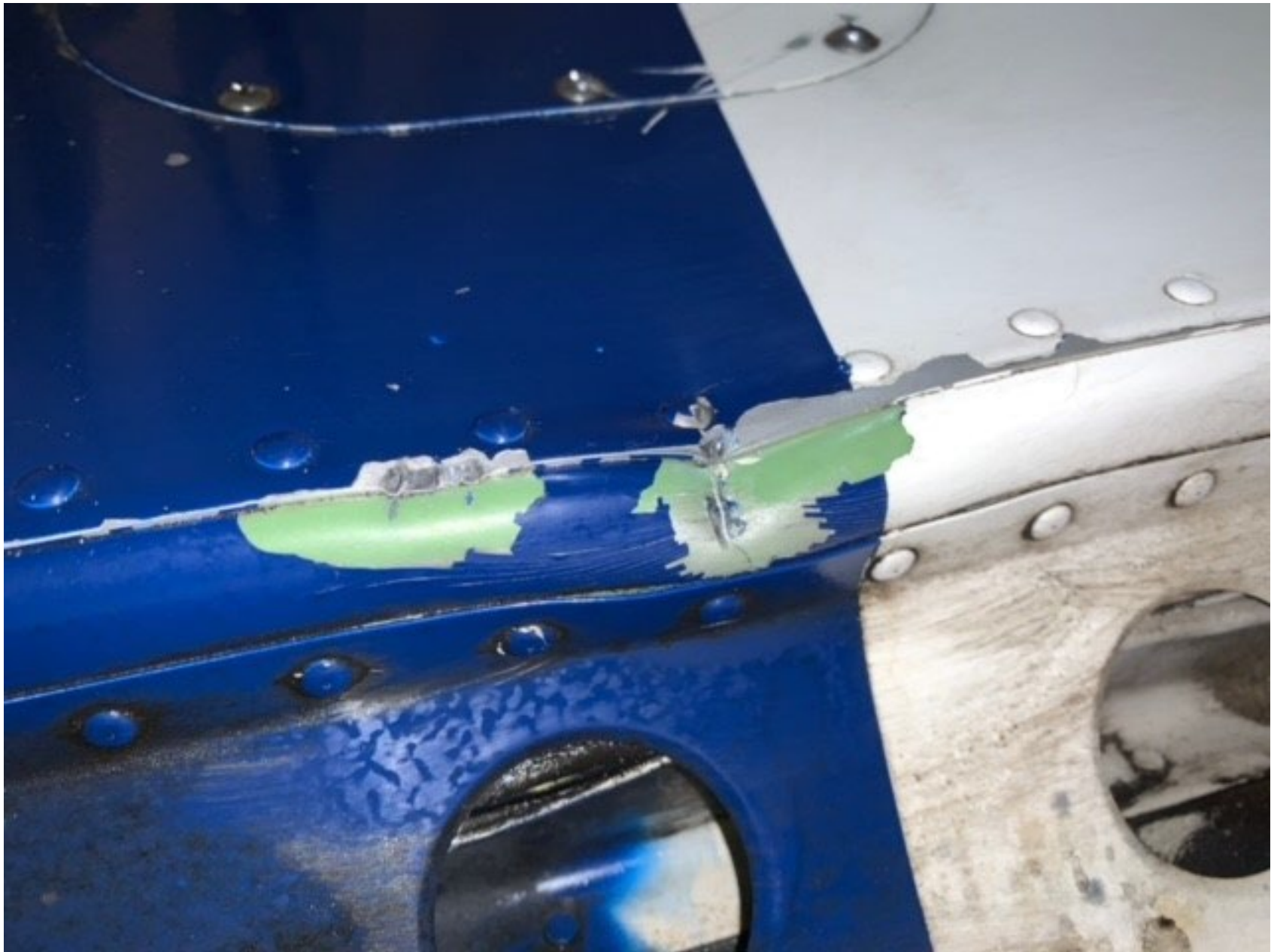
Photo 1 – Underside view of the right wing showing substantial damage. Photo courtesy of the operator.
