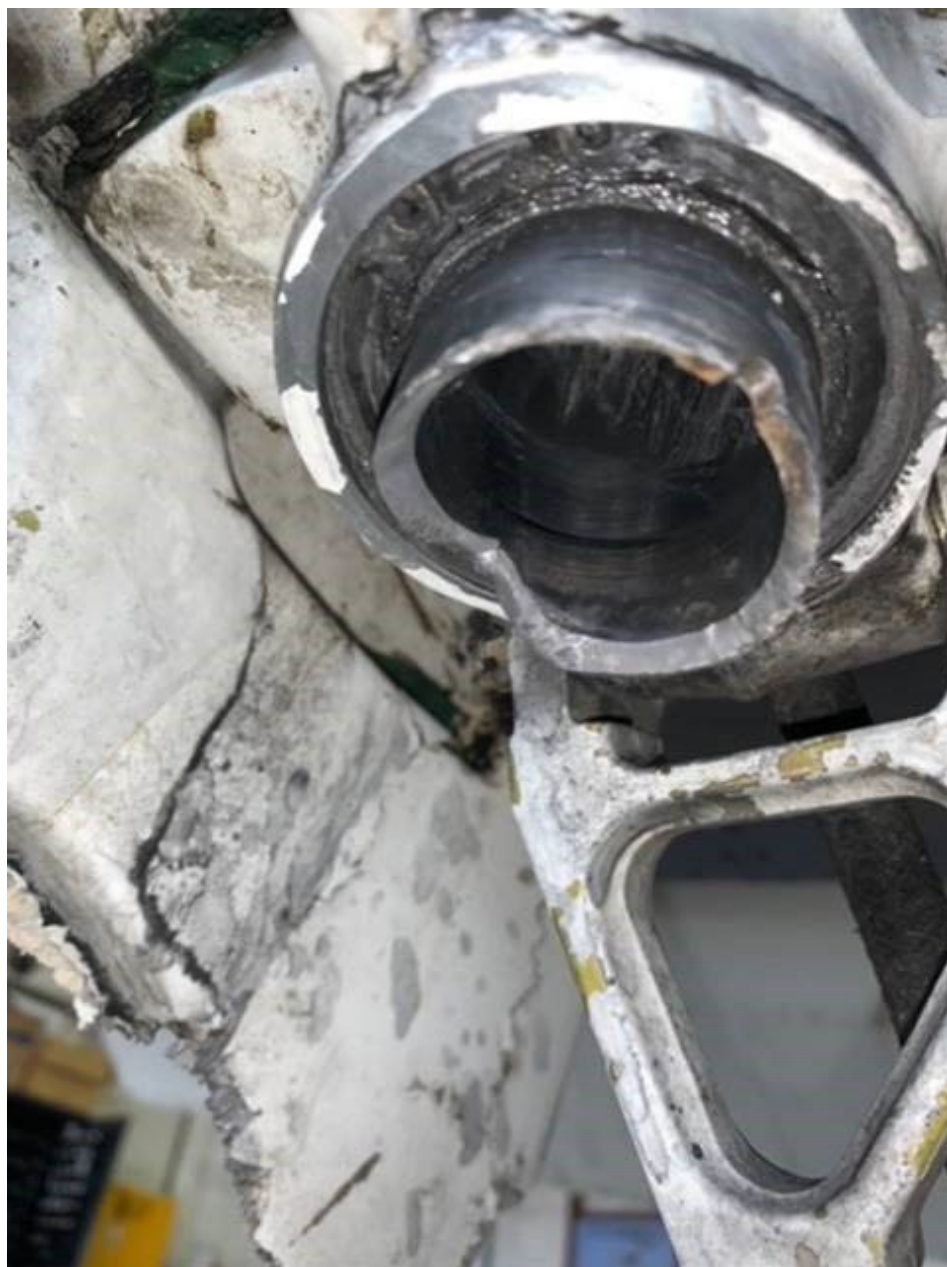
Photo 2 – View of the failed landing gear strut. Photo courtesy of the operator
