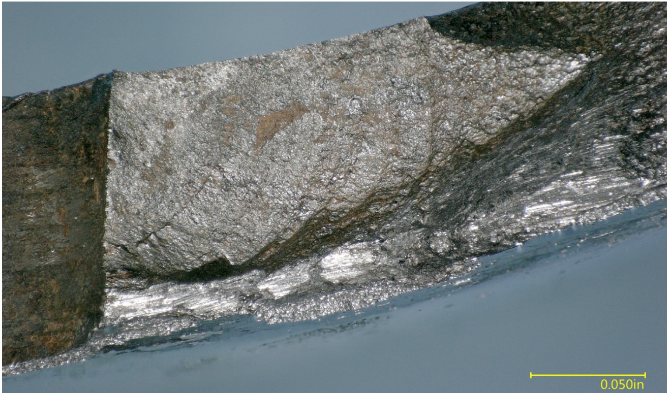
Figure 9 – View of the thumbnail crack on to the right of the hole in Figure 8.
