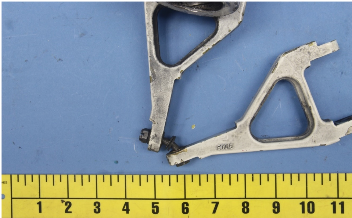
Figure 29 – View of a bent (but intact) attachment bolt connecting the two upper and lower torque links.
