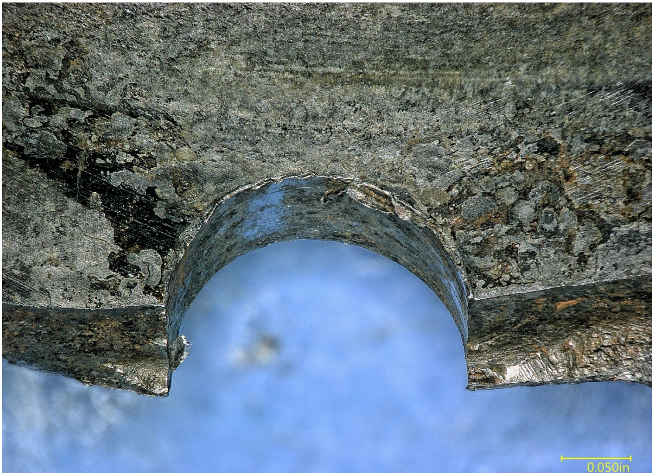
Figure 12 – Angled view showing the interior of the piston cylinder at the hole and cracks.
