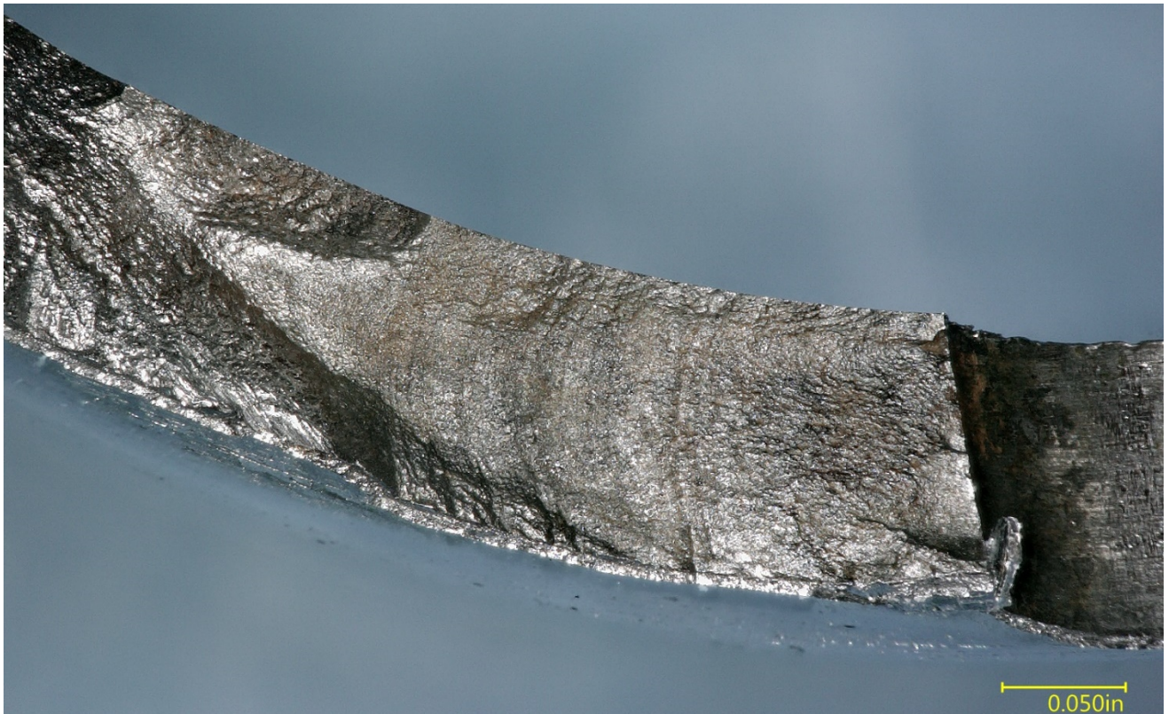
Figure 10 – View of the thumbnail crack on to the left of the hole in Figure 8.
