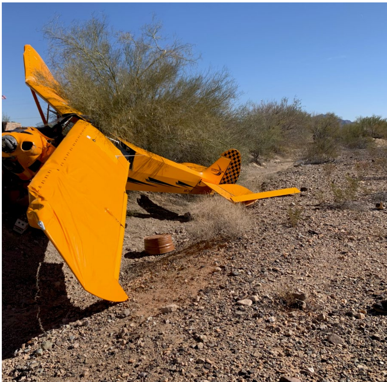
Photo 1 – View of damage to the left wing and right wing (Courtesy of Pilot)
