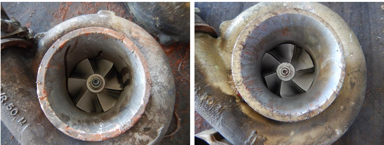
Figure 8-Turbocharger compressor scrolls and blades.
