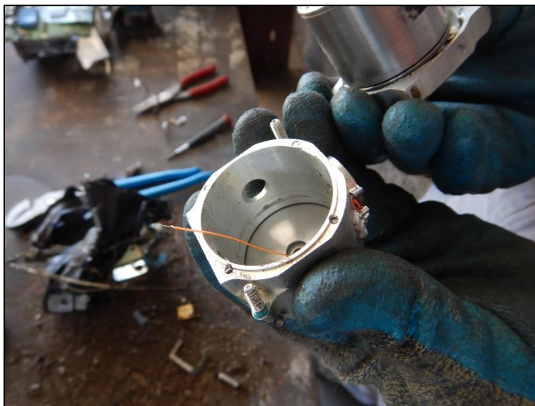
Figure 3-Attitude indicator case, interior rotational scoring.
