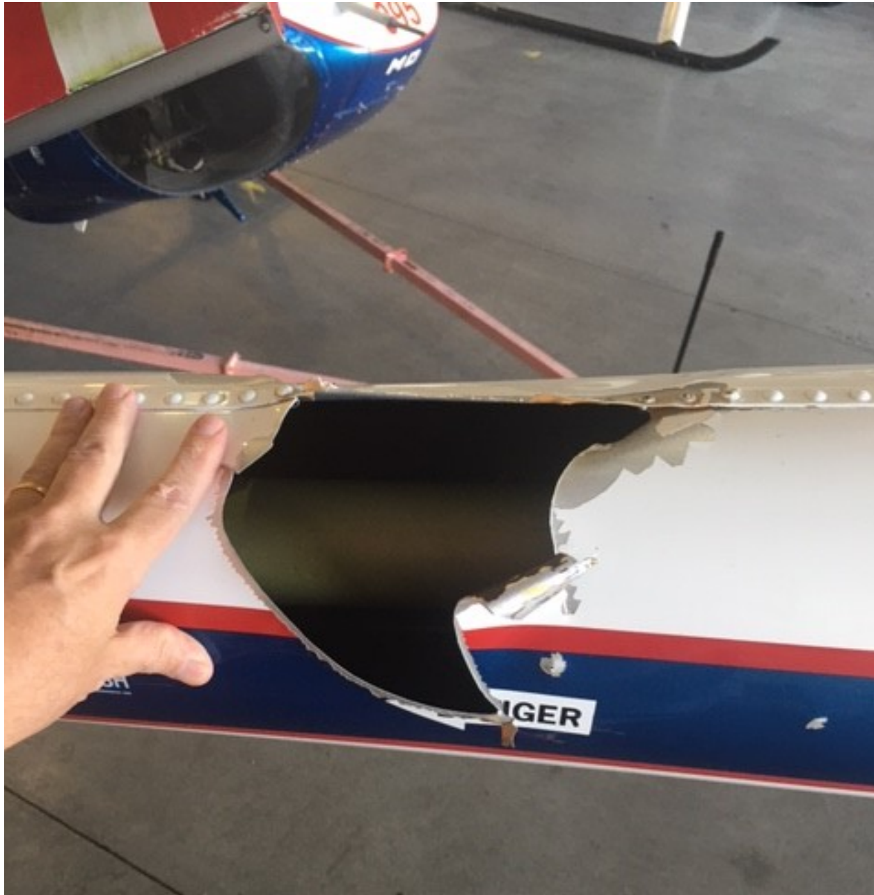
Photo 1 – Top view, showing damage to the tail boom. Photo courtesy of the operator.
