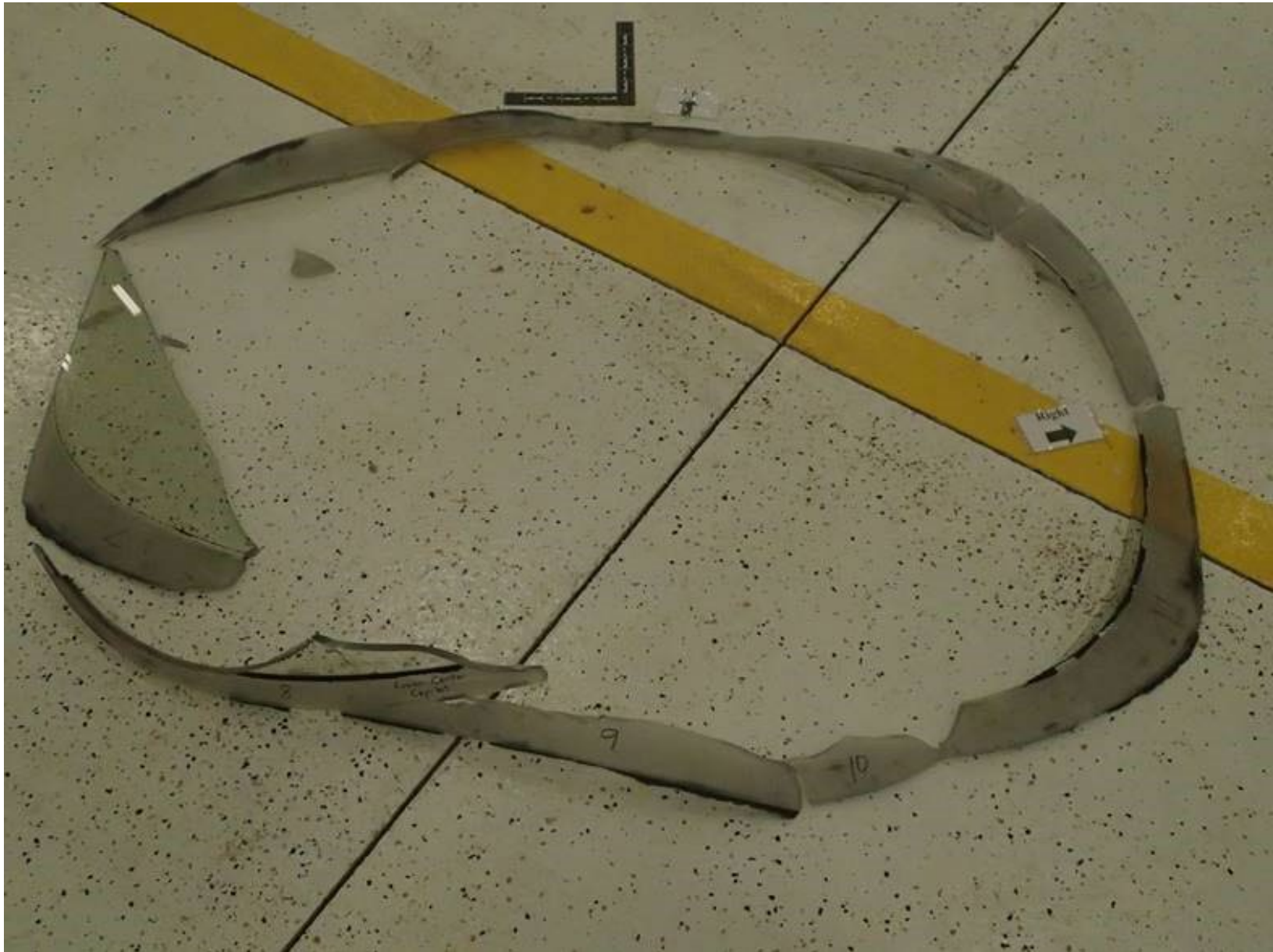
Photo 4 – Windshield as removed from fuselage (courtesy of witness)
