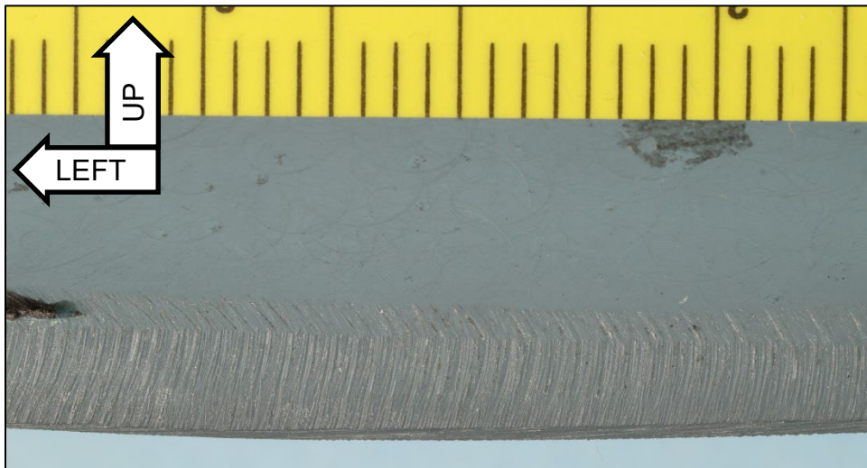
Figure 23. Linear grinding marks at the lower edge of piece 8 on the interior side of the windshield.
