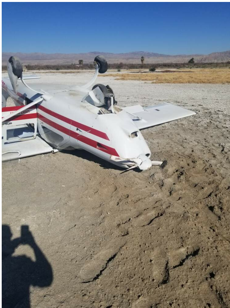
Photo 1 – View of substantial damage to the left wing at the forward upper fuselage wing root (Courtesy of Pilot)
