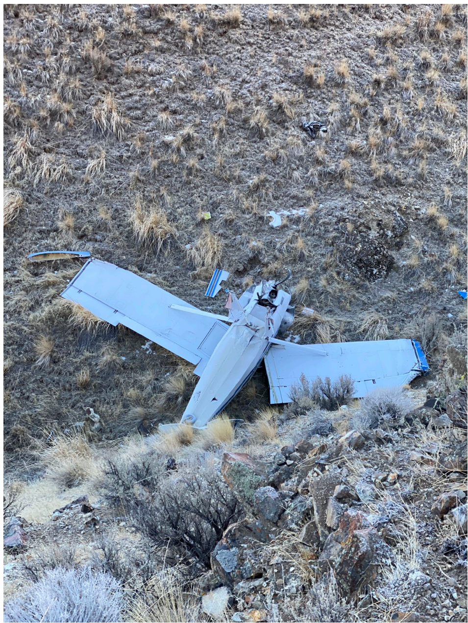
Photo 1 – View of inverted airplane with damaged left-wing (courtesy of the pilot)
