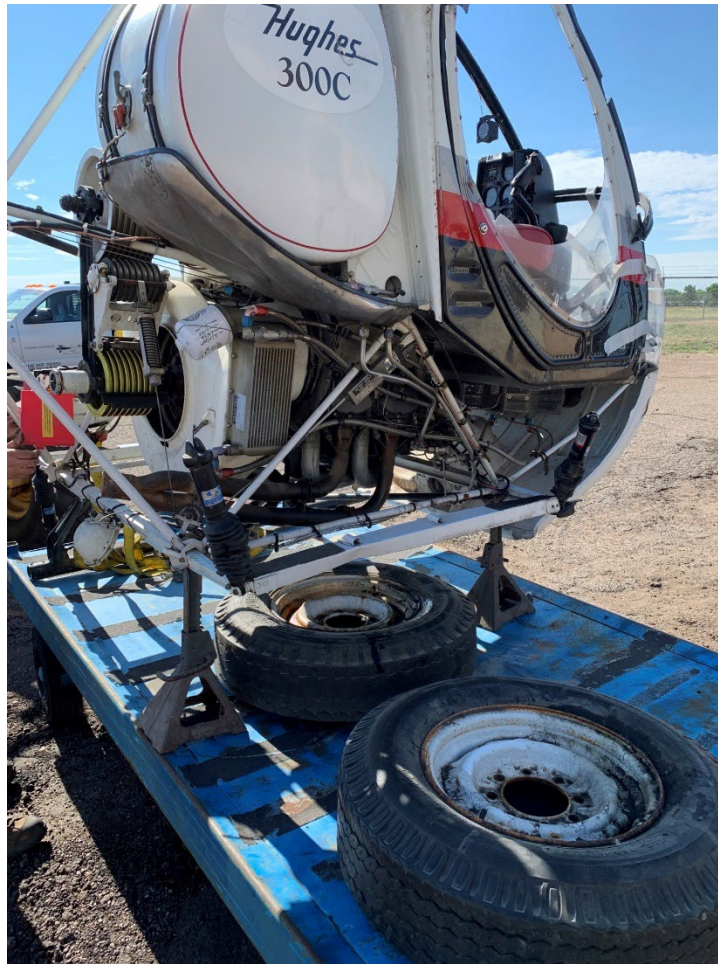
Figure 6, Helicopter Strapped to Trailer for Engine Run
