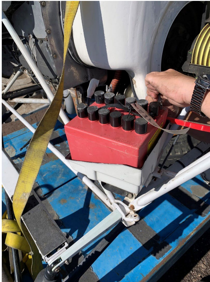
Figure 7, Installed 24-Volt Battery
