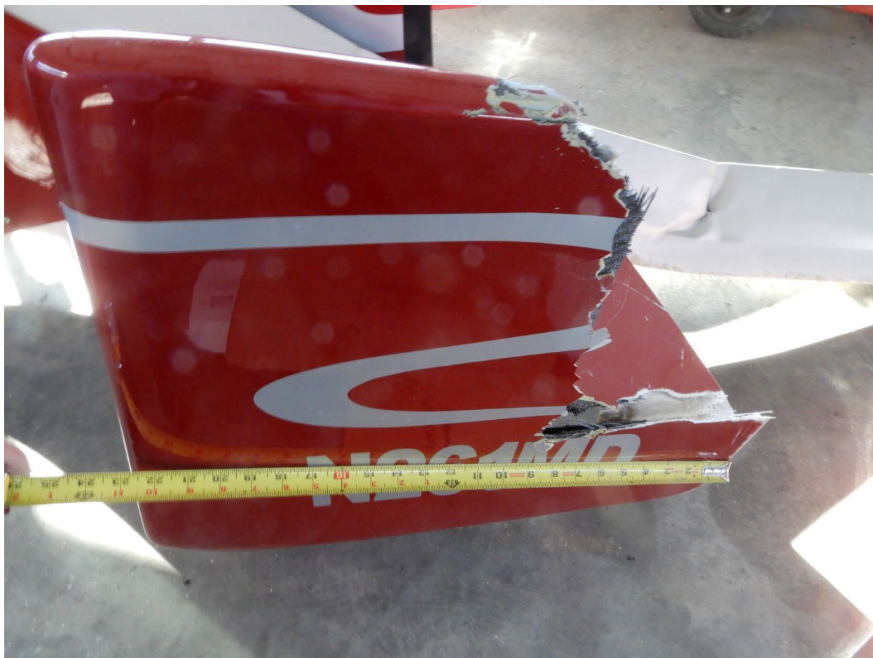
Figure 14. Left vertical stabilizer, showing damaged aft section.
