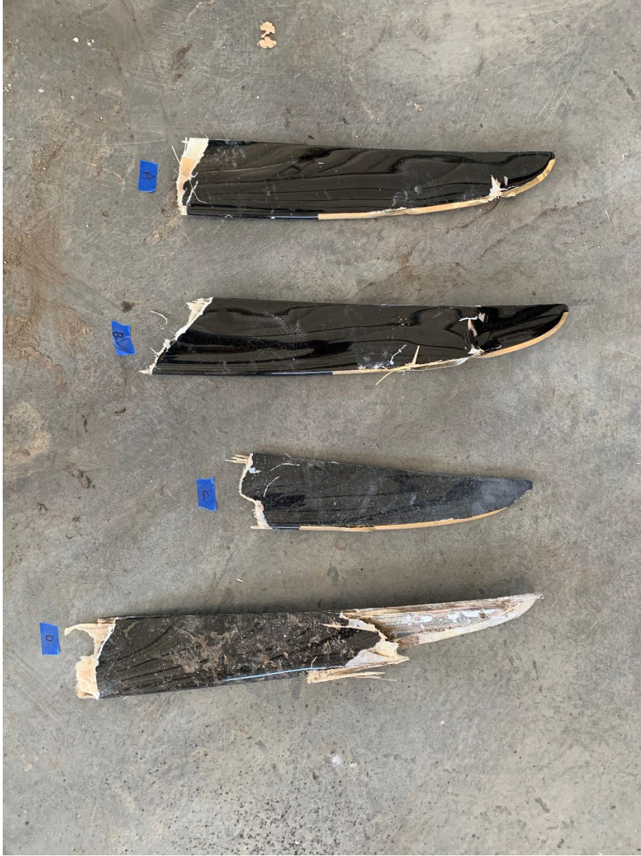
Figure 17. Propeller blade tips, other side, showing minor damage at the tips.
