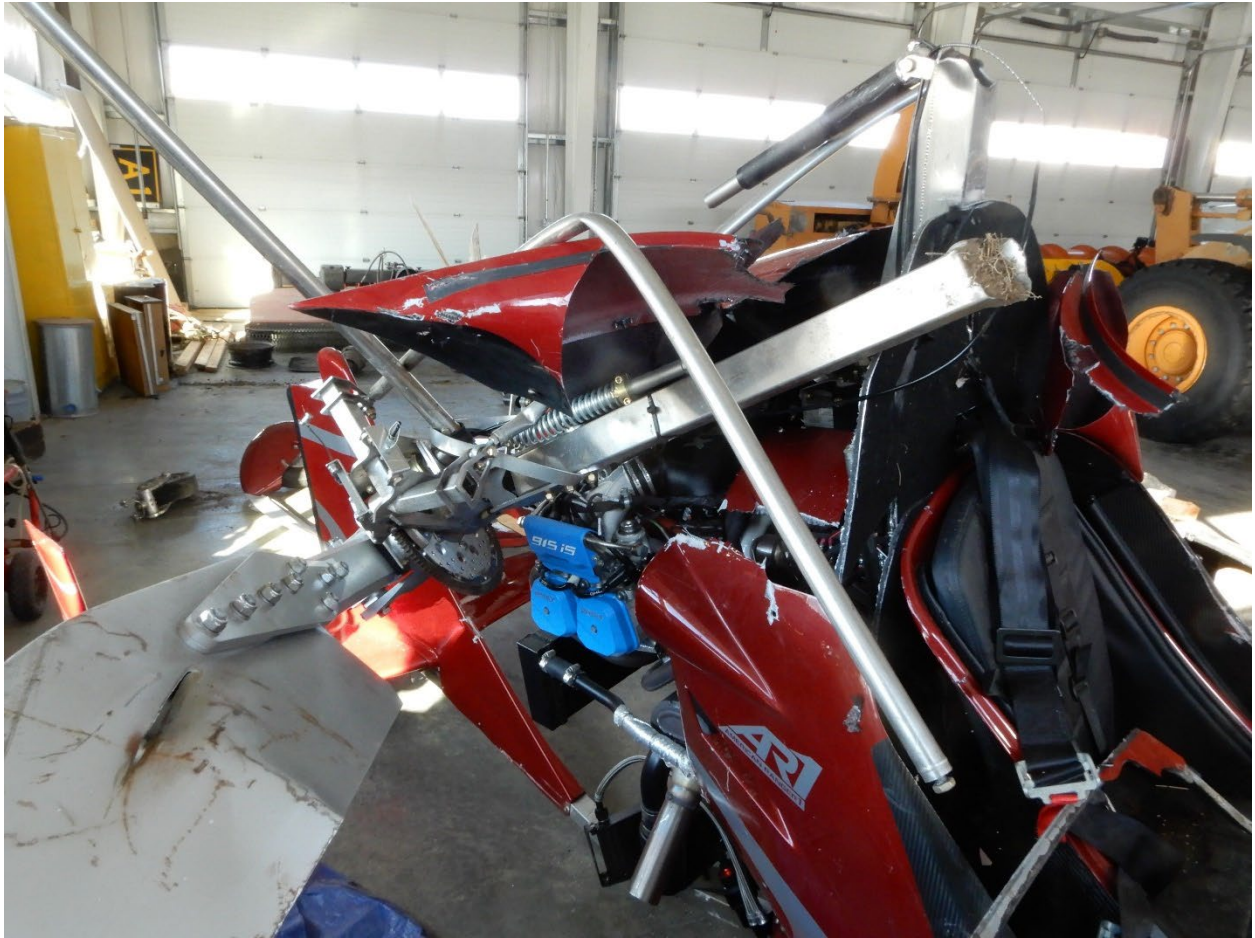
Figure 19. Right-side view, showing the rotor mast separation point.
