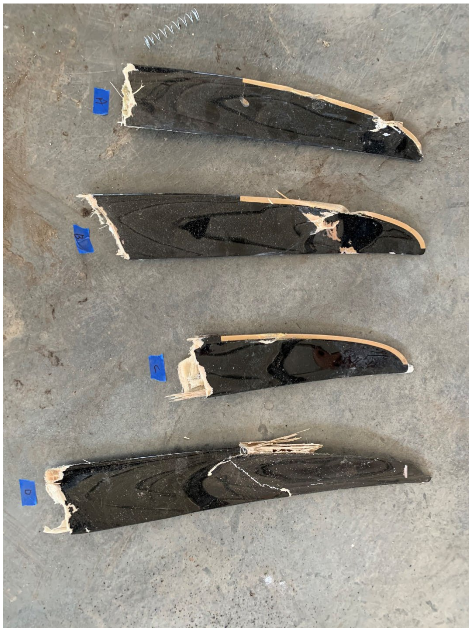
Figure 16. Propeller blade tips, showing minor damage at the tips.
