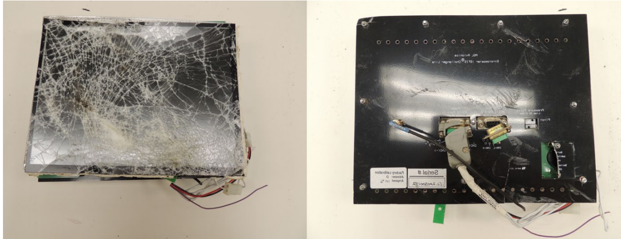
Figure 1. Front and back of MGL Avionics Challenger Lite as received.
