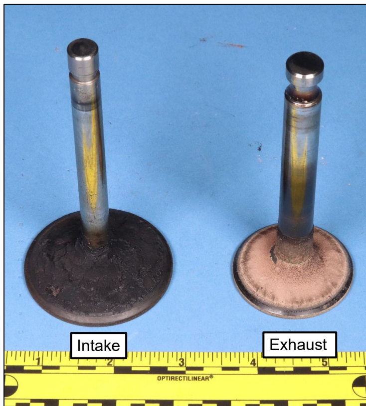
Figure 8. Intake and exhaust valves after removal from the cylinder assembly.
