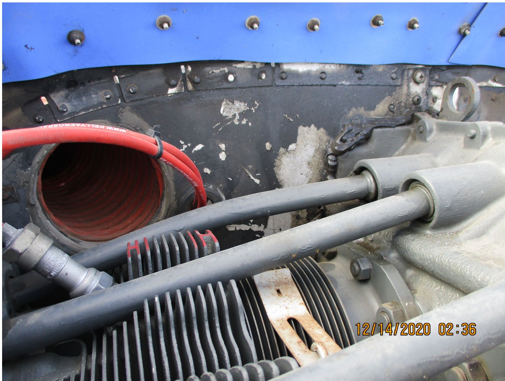
Photo 3 – View of the bent push rod tub on the number 3 cylinder (photo courtesy of the FAA)
