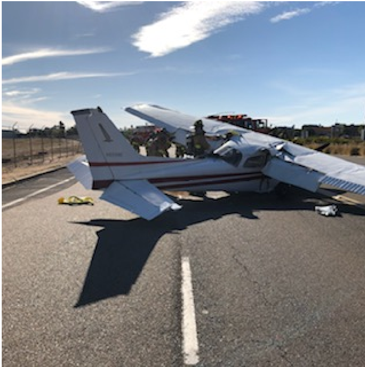
Photo 1 – View of left and right wing damage (photo courtesy of the FAA)
