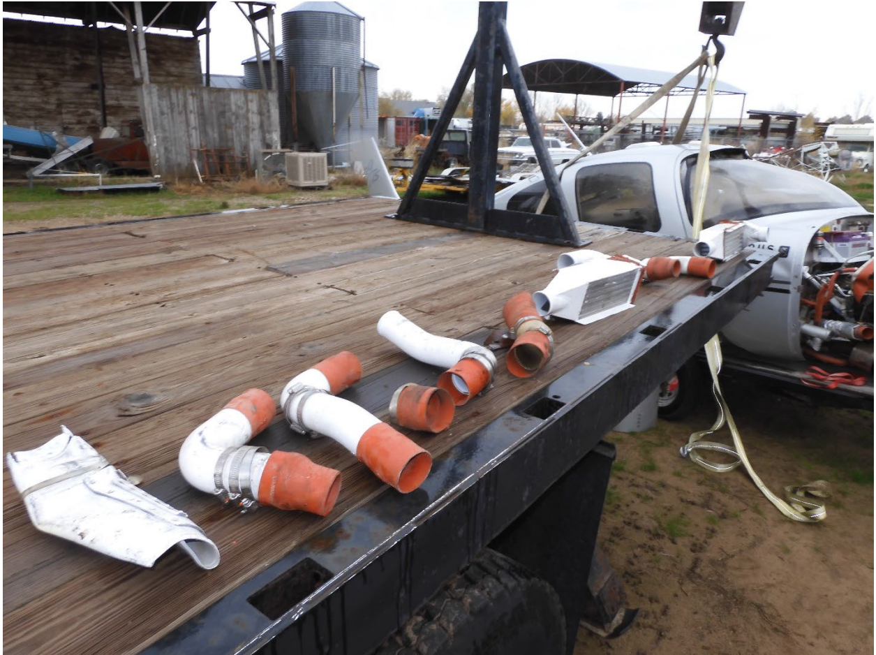
Figure 8. Air induction tubes, intercoolers, and sleeves removed.
