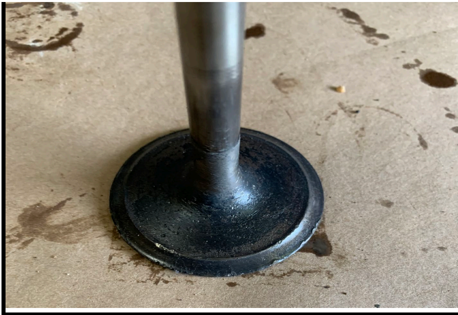
Figure 13: View of Cylinder #5 Intake Valve damage
