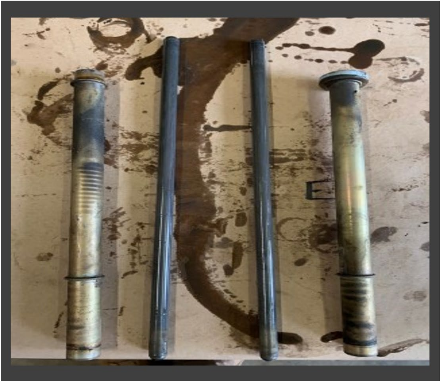
Figure 8: View of No. 2 push rods and housings
