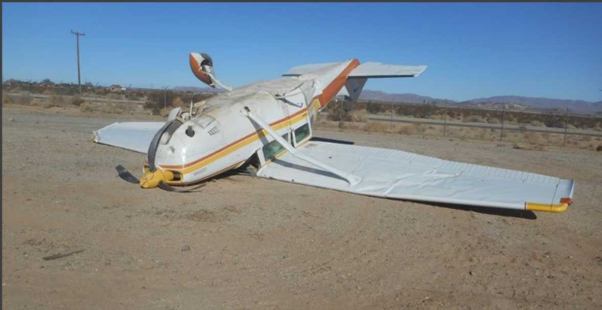
Figure 1: View of propeller damage which occurred upon impact with terrain
