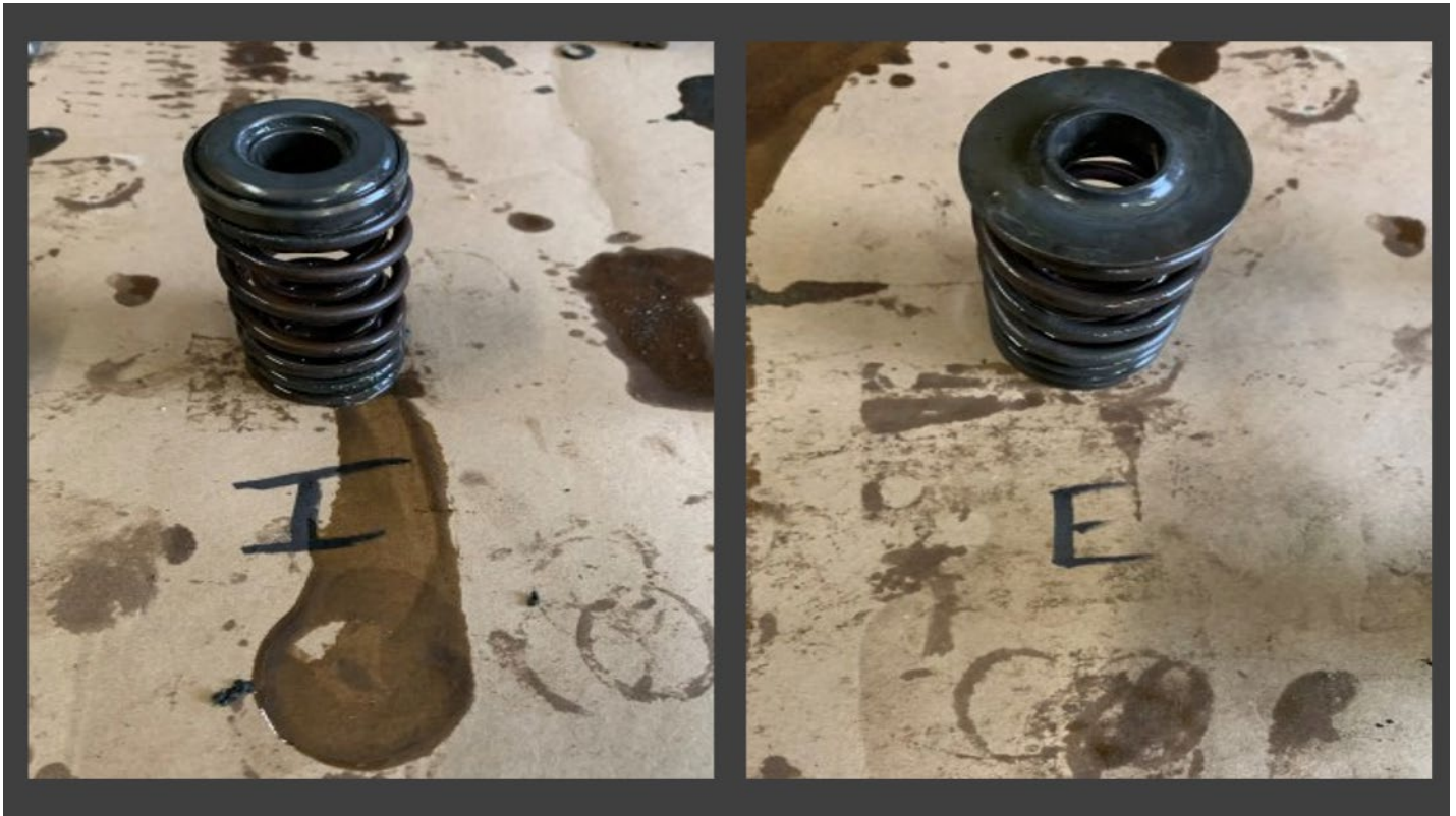
Figure 9: View of No. 2 intake & exhaust springs with seats
