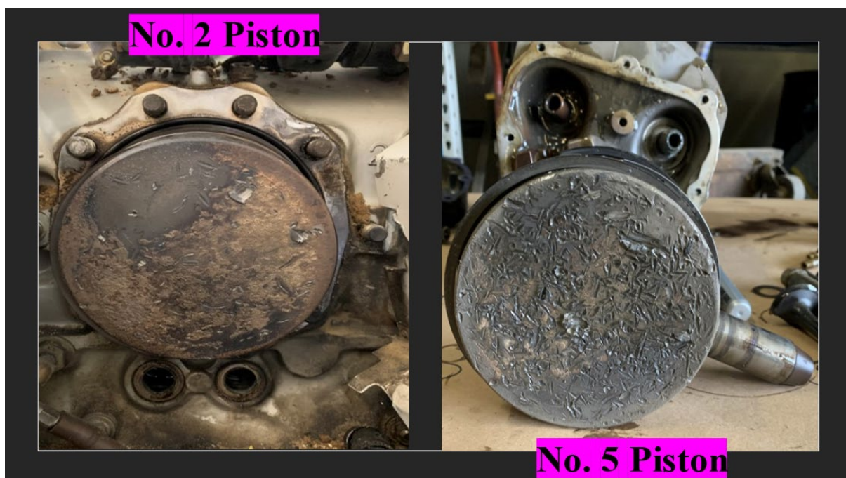
Figure 6: View of damage to No. 2 and No. 5 Pistons
