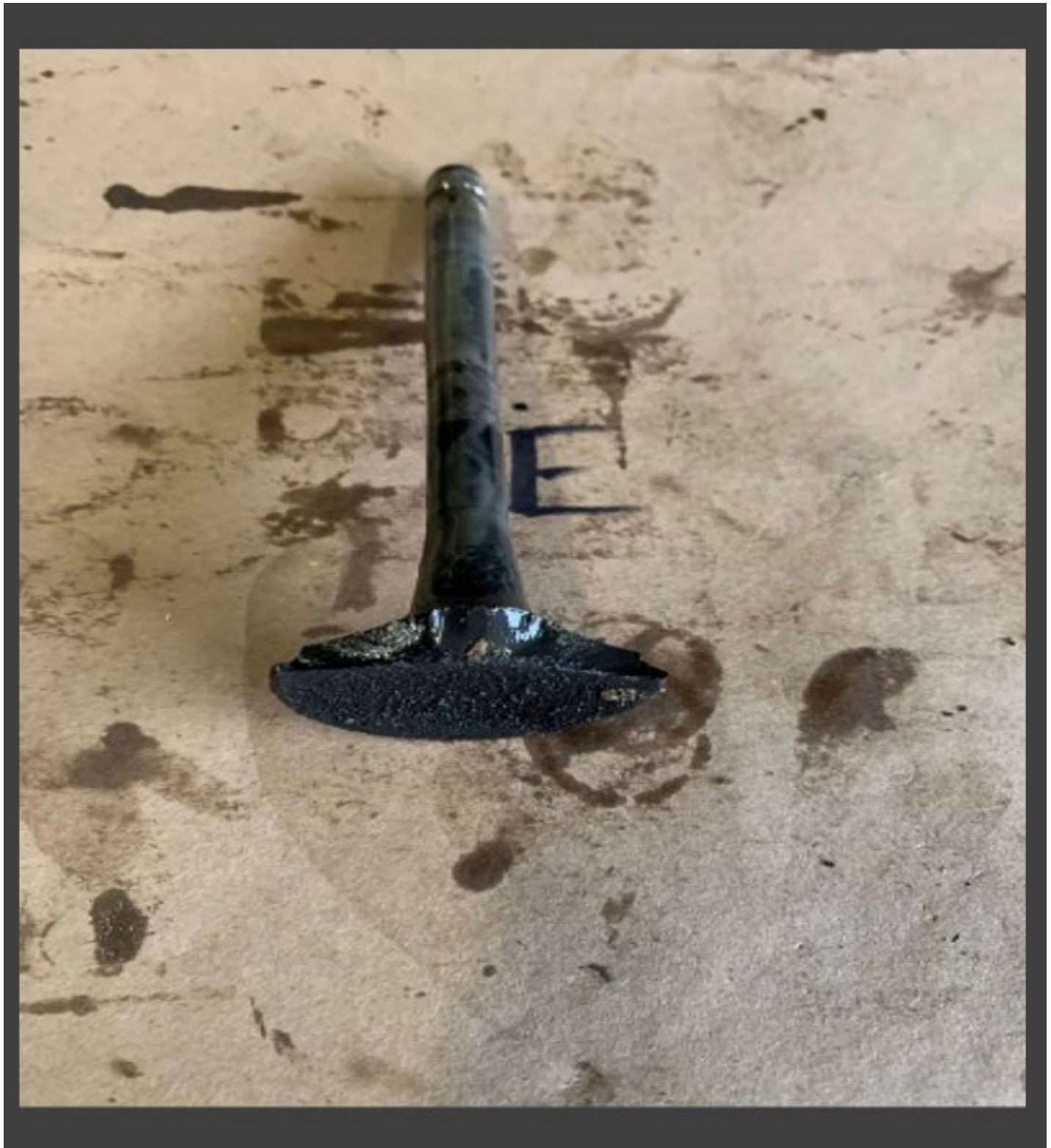
Figure 11: Profile view of No. 2 exhaust valve
