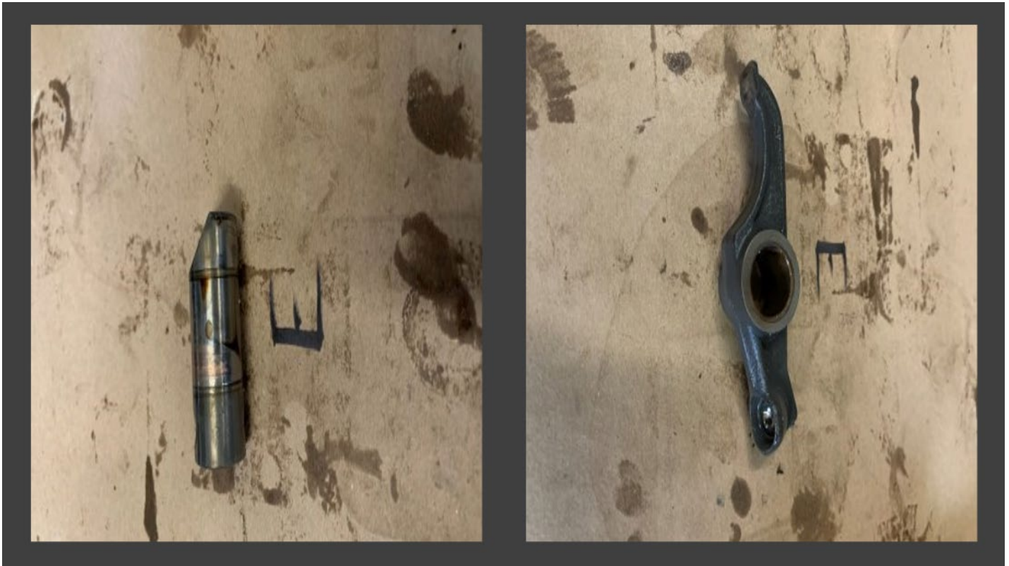
Figure 12: View of No. 2 cylinder exhaust rocker arm & shaft
