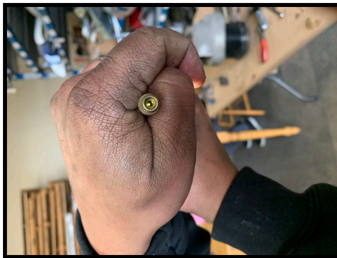
Figure 7: The No. 2 injector nozzle contained a greenish-yellowish foreign substance
