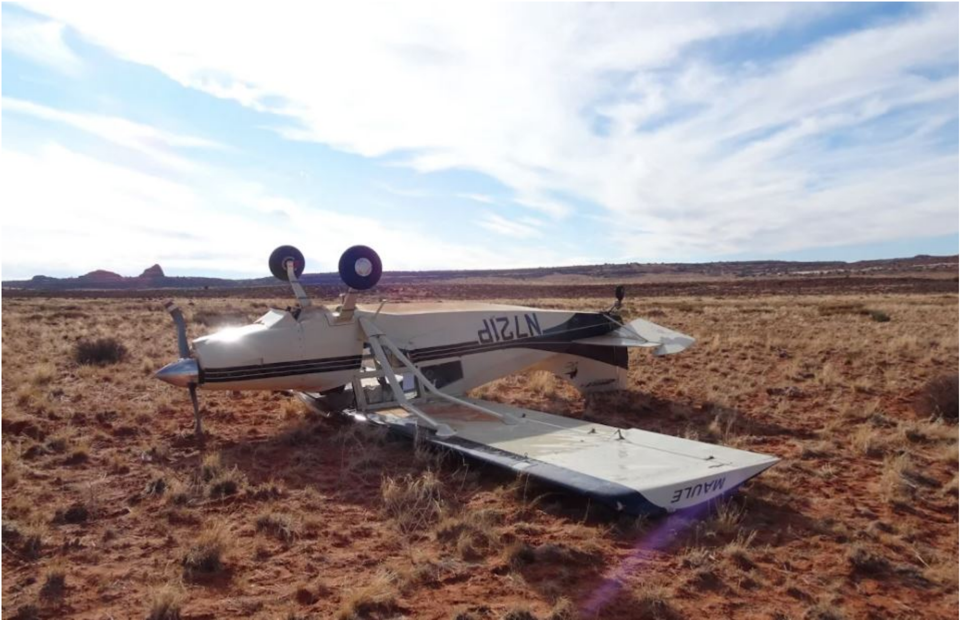
Photo 1 – View of nosed over airplane with damaged right-wing lift struts and rudder (courtesy of the FAA)
