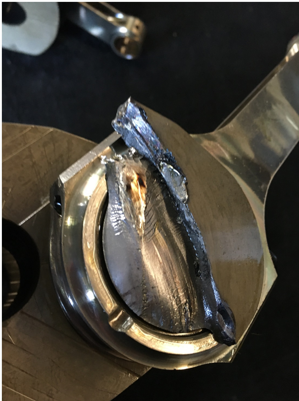
Photo 10 – N975G Broken Crankshaft, courtesy FAA FSDO
