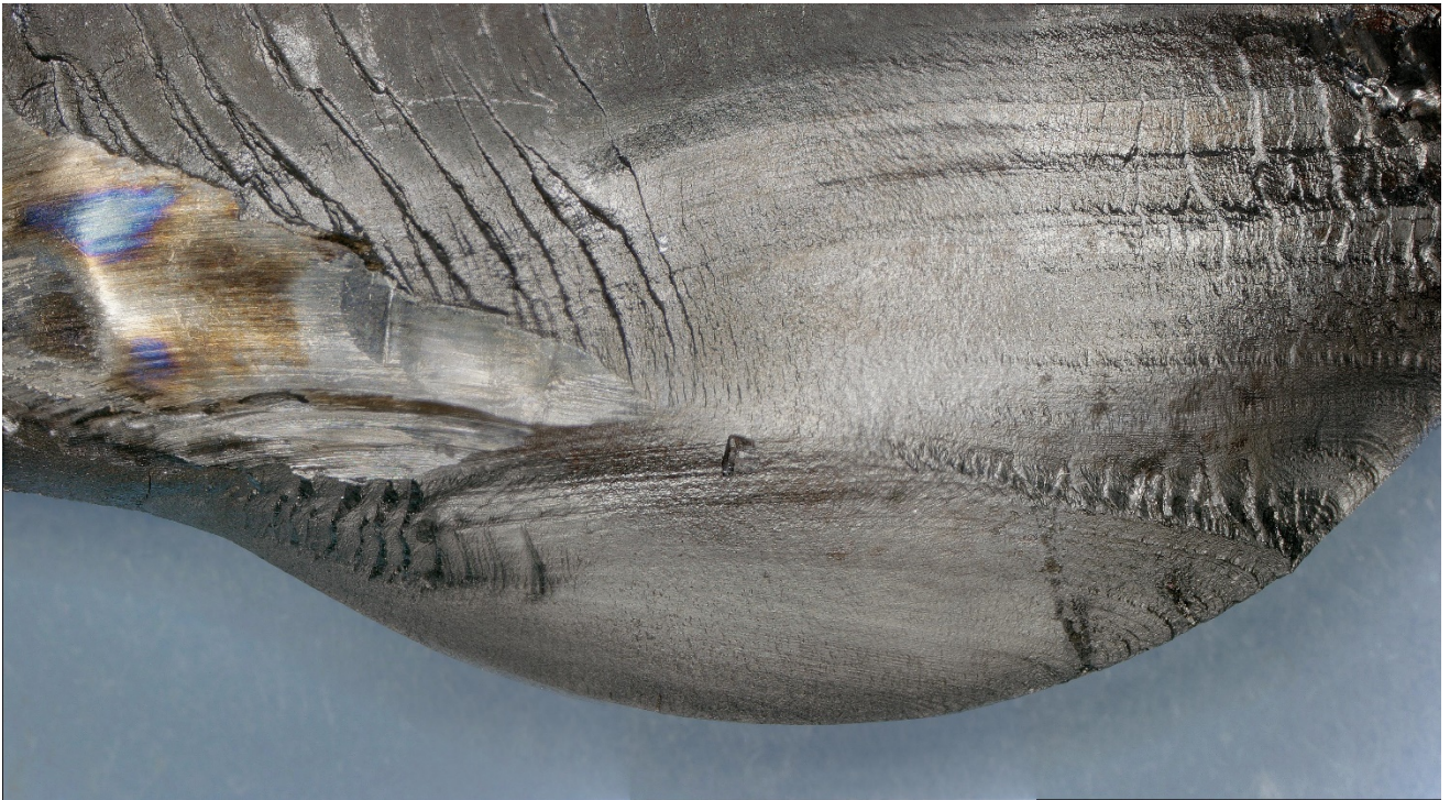
Figure 3 – Closer view of the forward mating fracture surface, after sectioning and cleaning.
