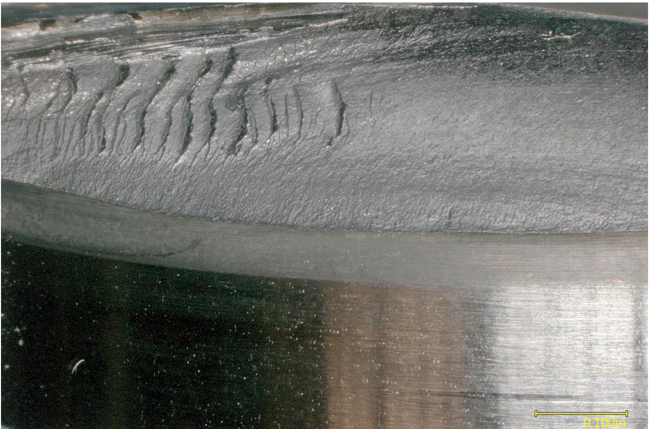
Figure 4 – View of the journal surface adjacent to the crack initiation sites of the fracture.
