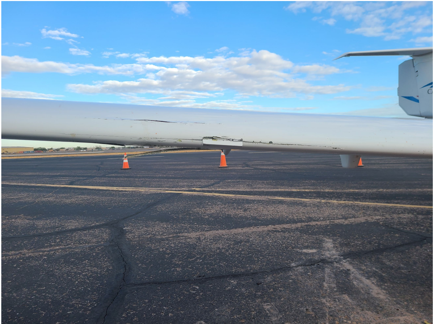
Photo 1 – photo of damage to leading edge of right wing (courtesy of CAE Aviation Academy)
