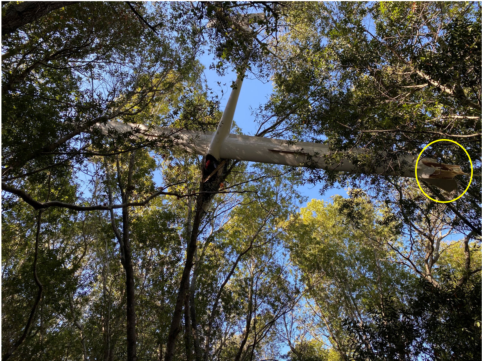
Photo 3 – N18MA view of left wing damage (photo courtesy of the FAA)
