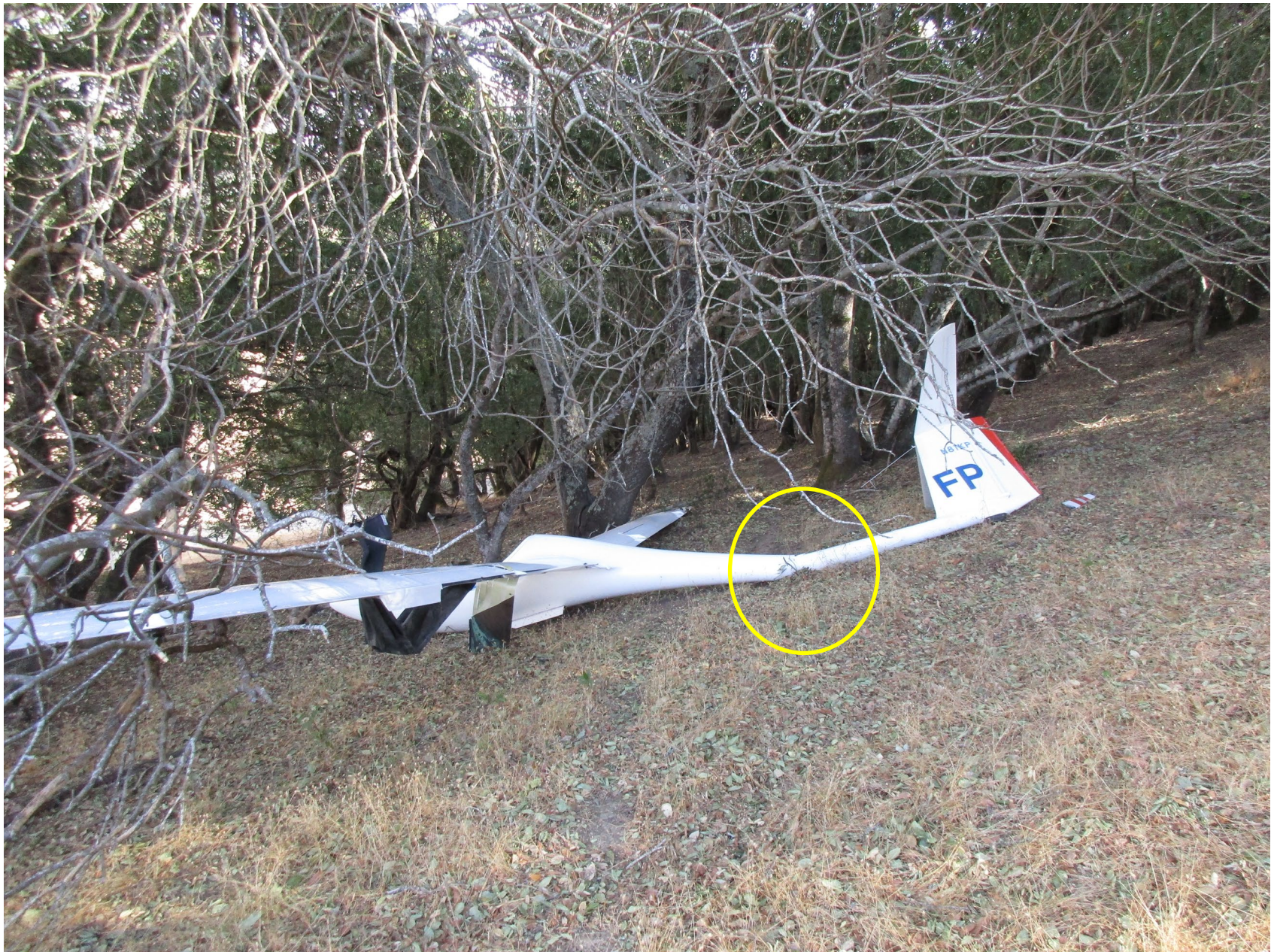
Photo 2 – N81KP view of aft fuselage damage (photo courtesy of the FAA)
