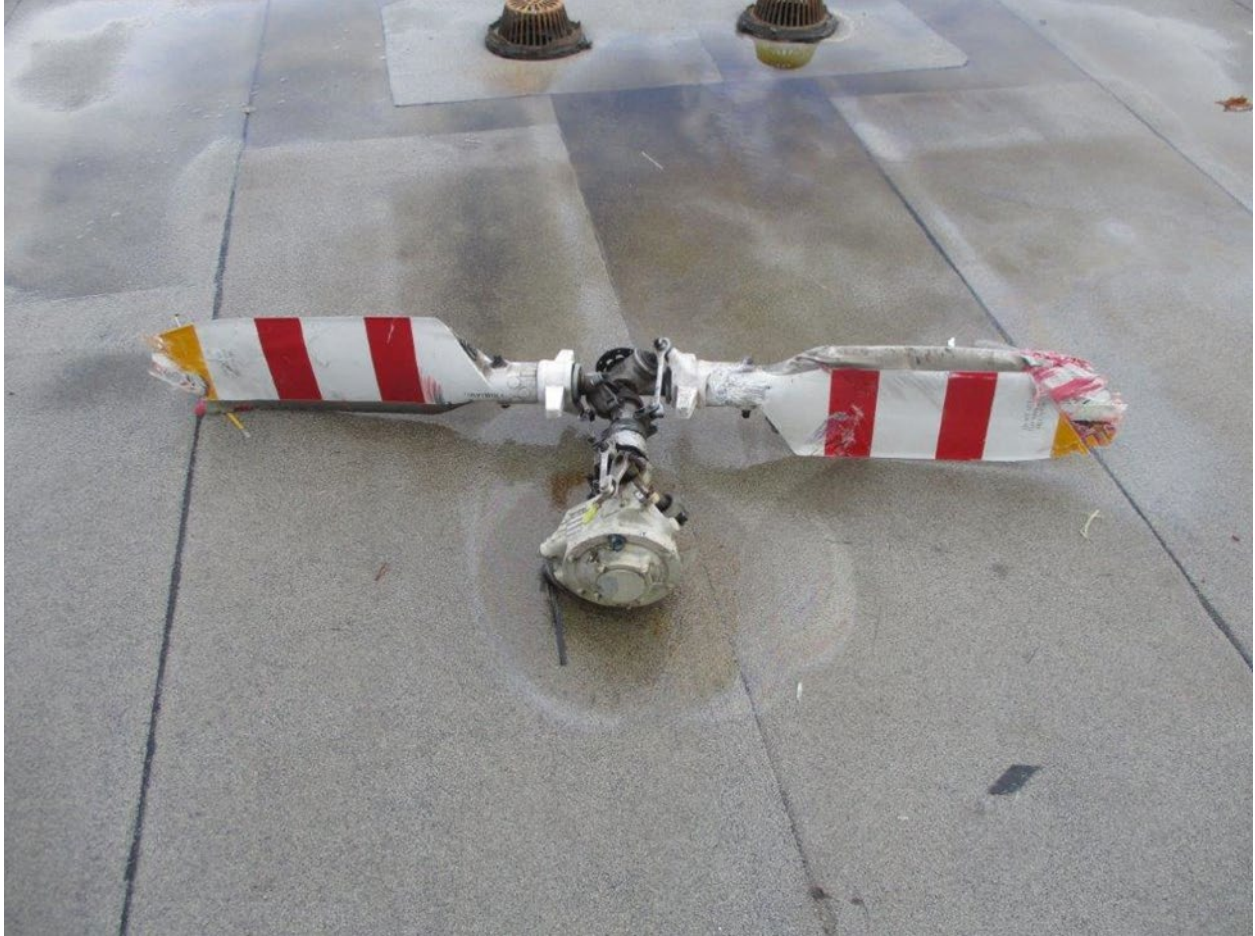
Figure 11. Tail rotor assembly and 90° gear box, Photo courtesy of the recovery agent.
