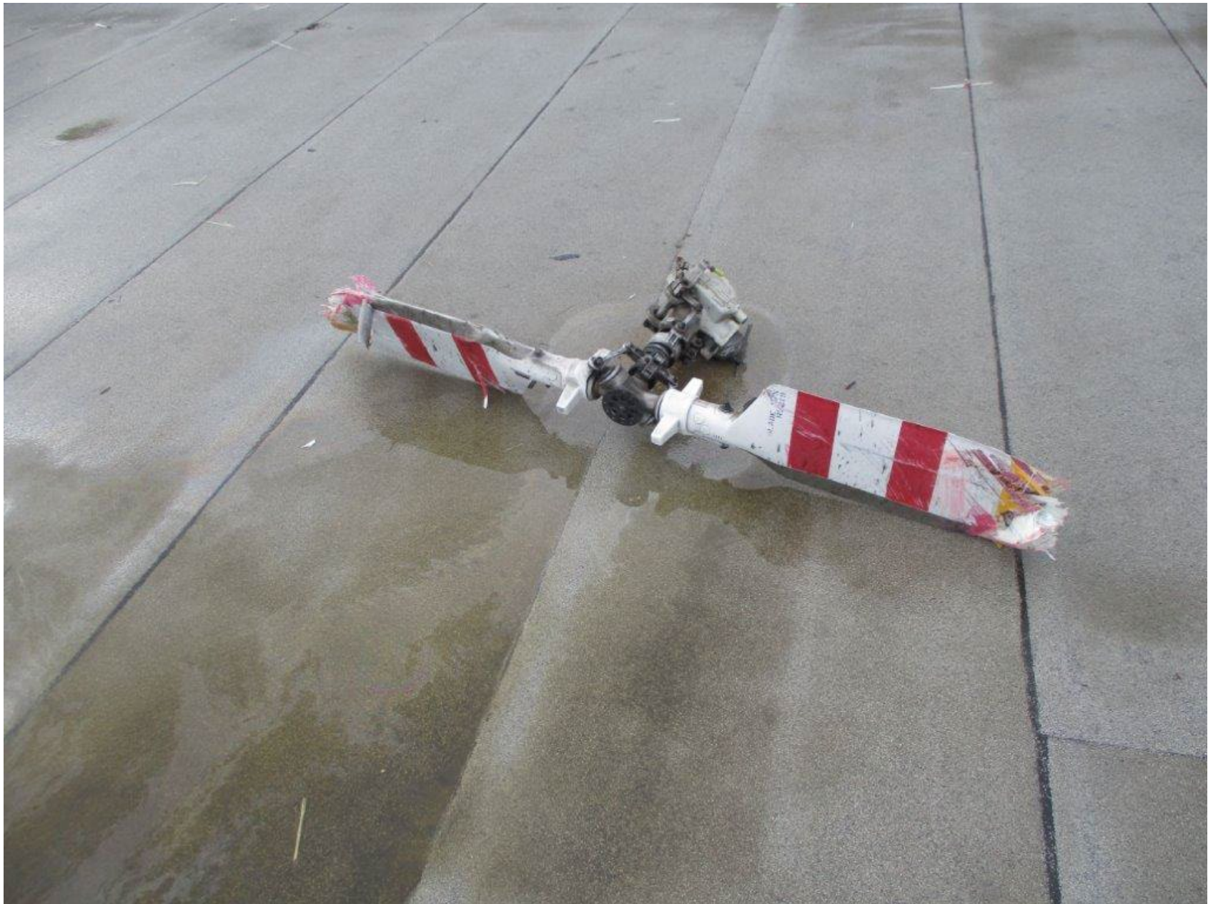
Photo 6 – Tail rotor assembly and 90-degrees gearbox. Photo courtesy of the operator.
