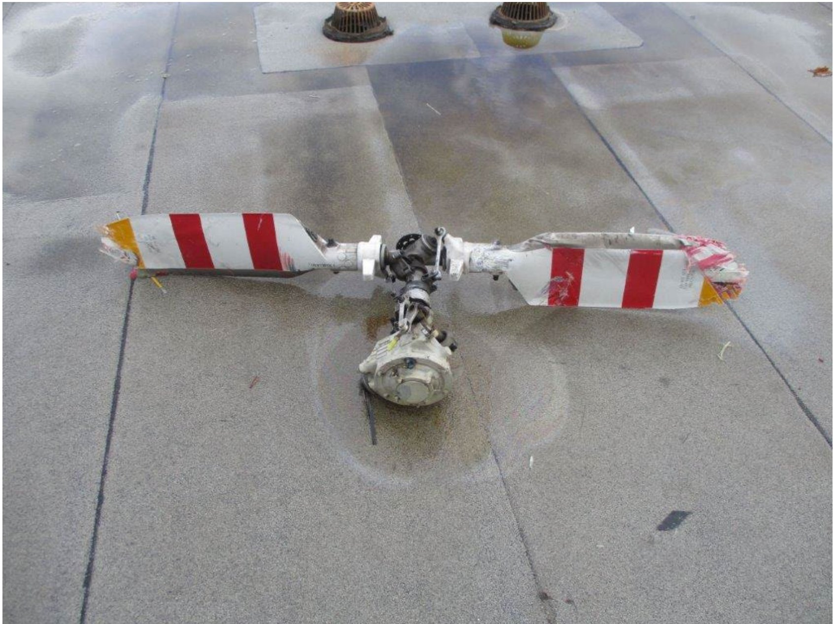
Photo 5 – Tail rotor and 90-degrees gearbox. Photo courtesy of the operator.
