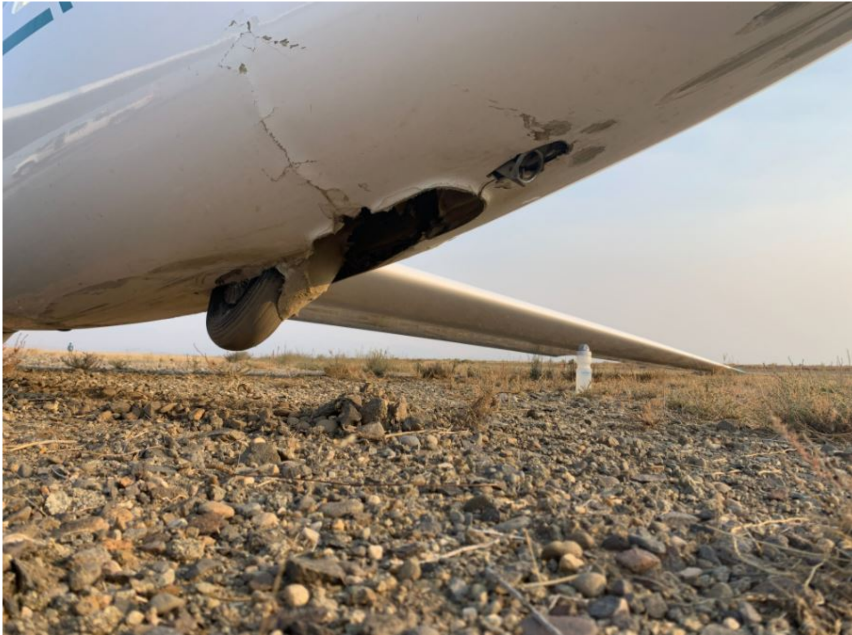
Photo 1 – View of damaged fuselage (courtesy of the FAA)
