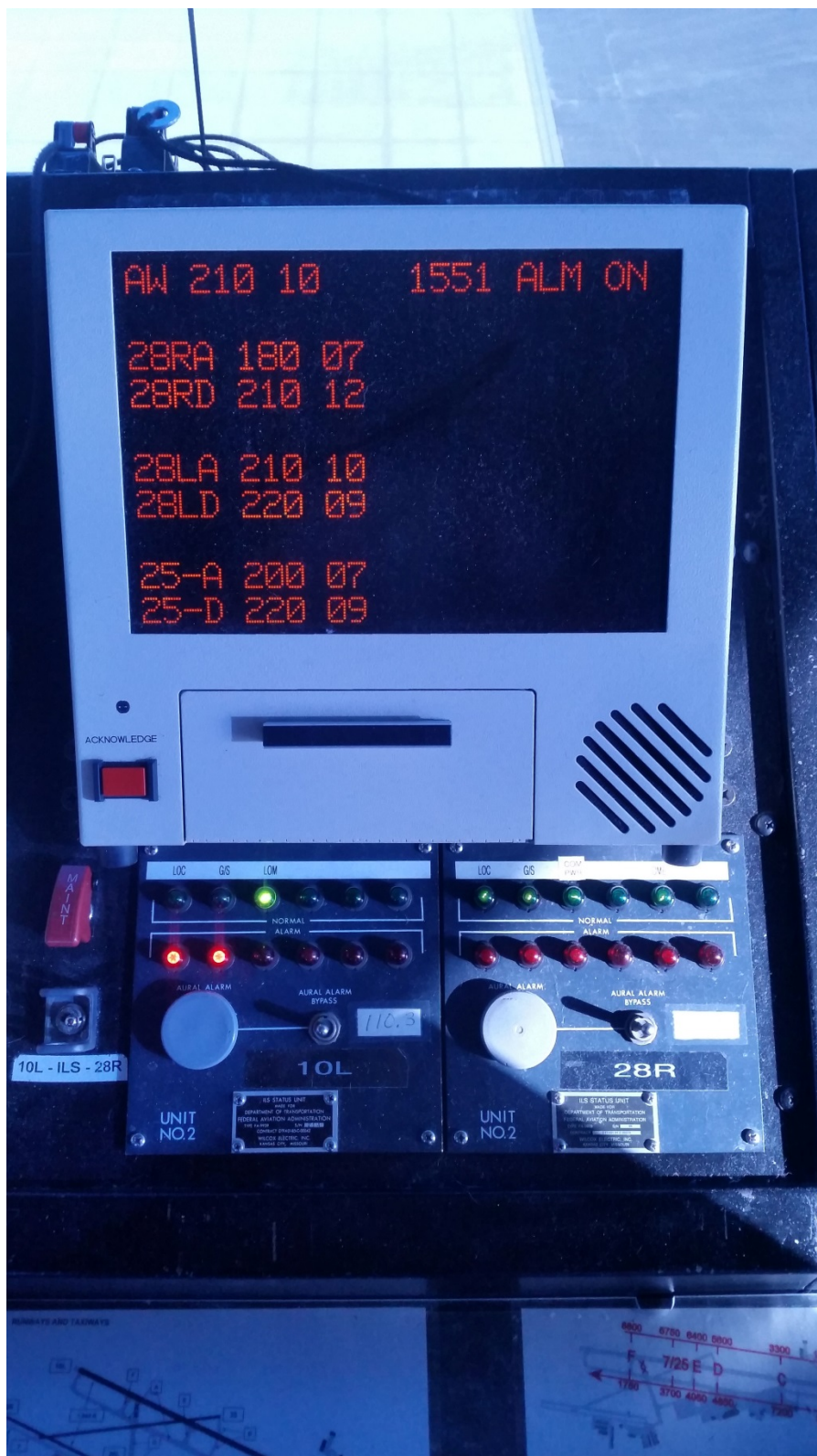
Figure 11 – Example of the LLWAS display for the Billings ATC
