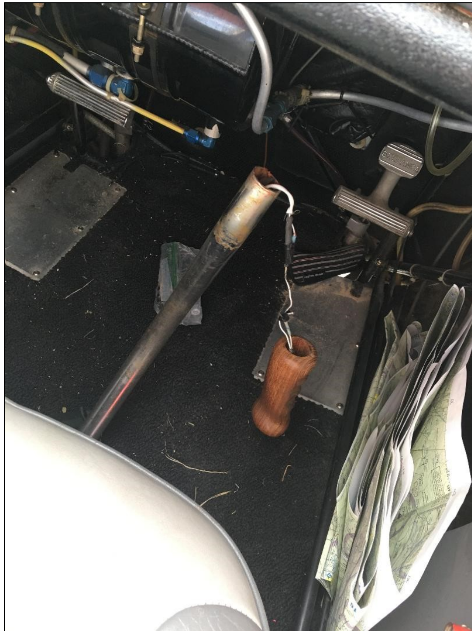
Photo 4 - Cabin area, with wood grip separated from control column.
