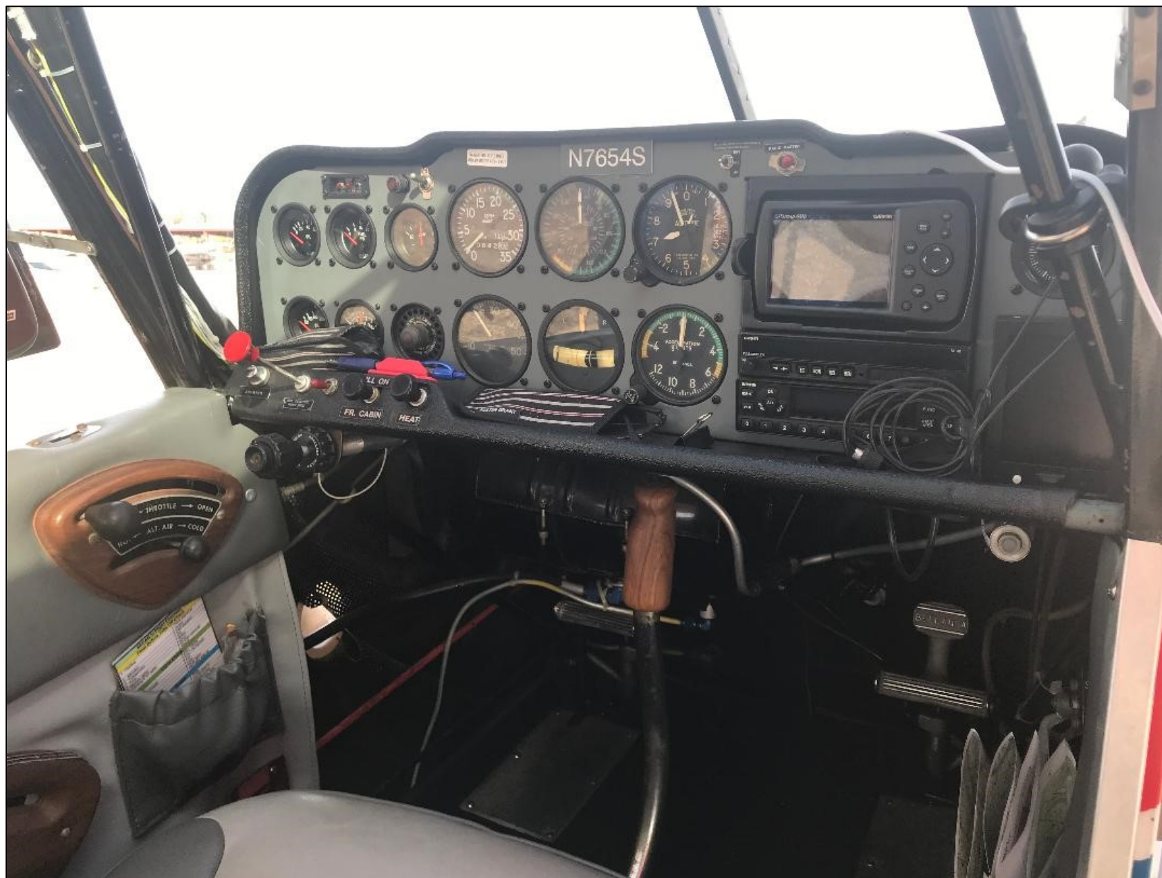
Photo 2 - Cabin area, with wood grip installed on the control column.
