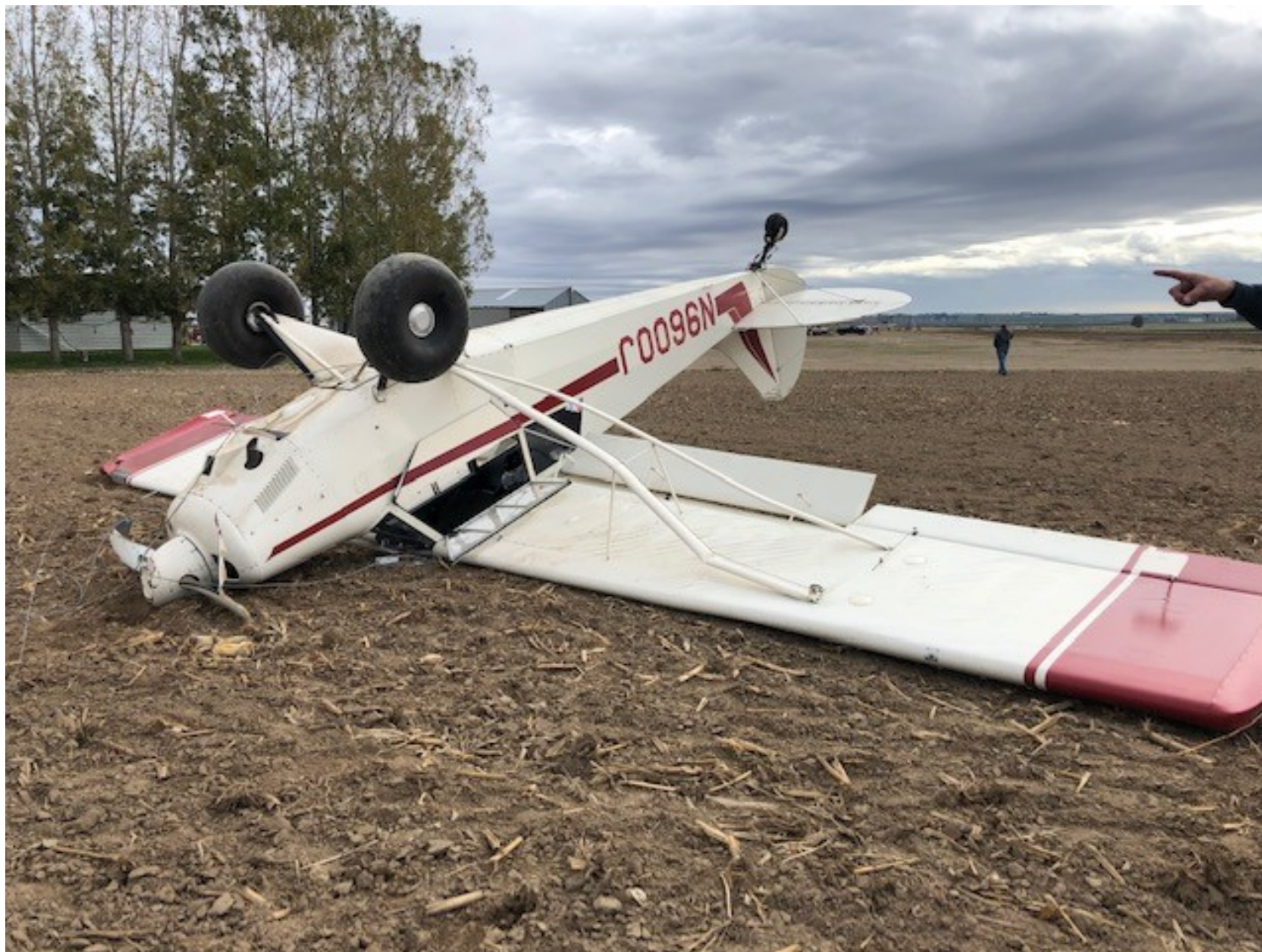
Photo 1 – View of nosed over airplane with damaged right wing lift strut and rudder (courtesy of the pilot)
