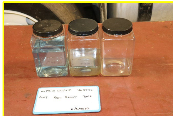
Figure 5. Total liquid drained from the right fuel tank
