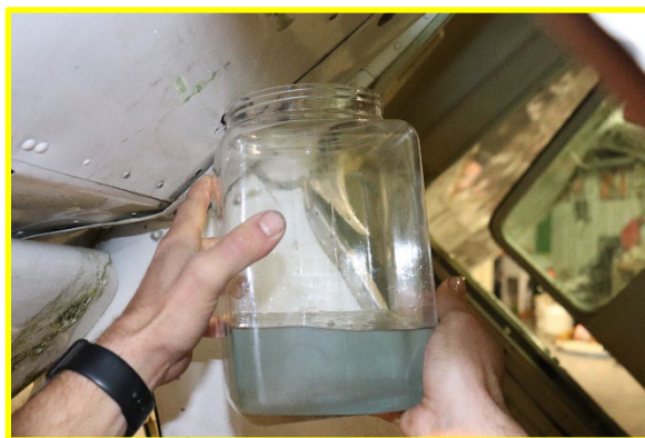
Figure 4. A portion of liquid drained from right fuel tank
