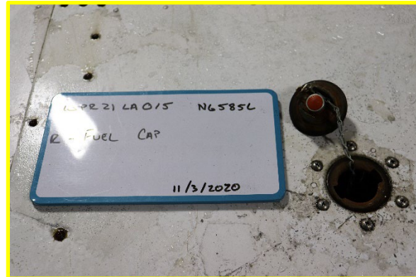
Figure 3. View of right fuel cap
