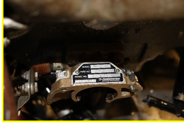
Figure 9. Carburetor impact separated at the mount
