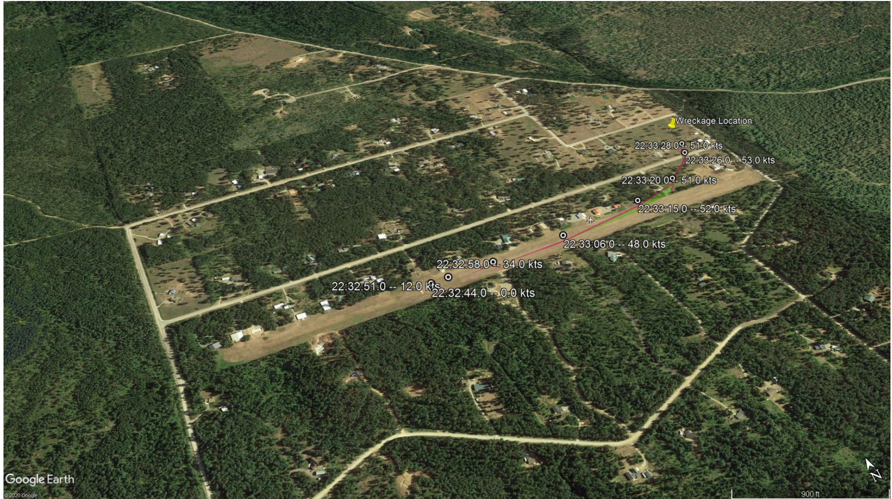
Figure 2. Google Earth overlay showing the accident flight and recorded groundspeed.
