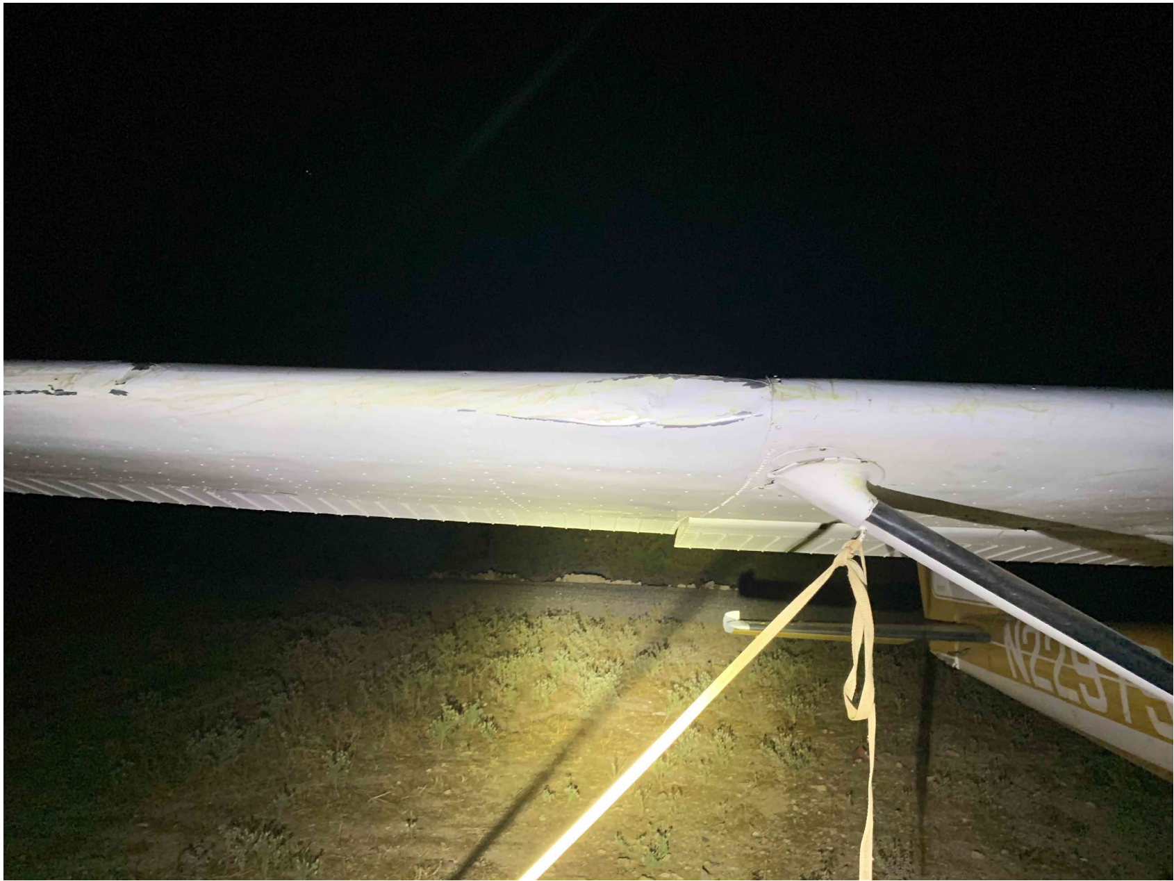
Photo 1 – view of damage to leading edge of right wing (photo courtesy of Yavapai Sheriff's Department)
