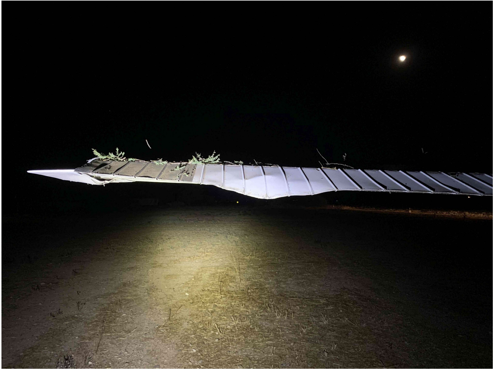
Photo 2 – view of damaged left aileron (photo courtesy of Yavapai Sheriff's Department)
