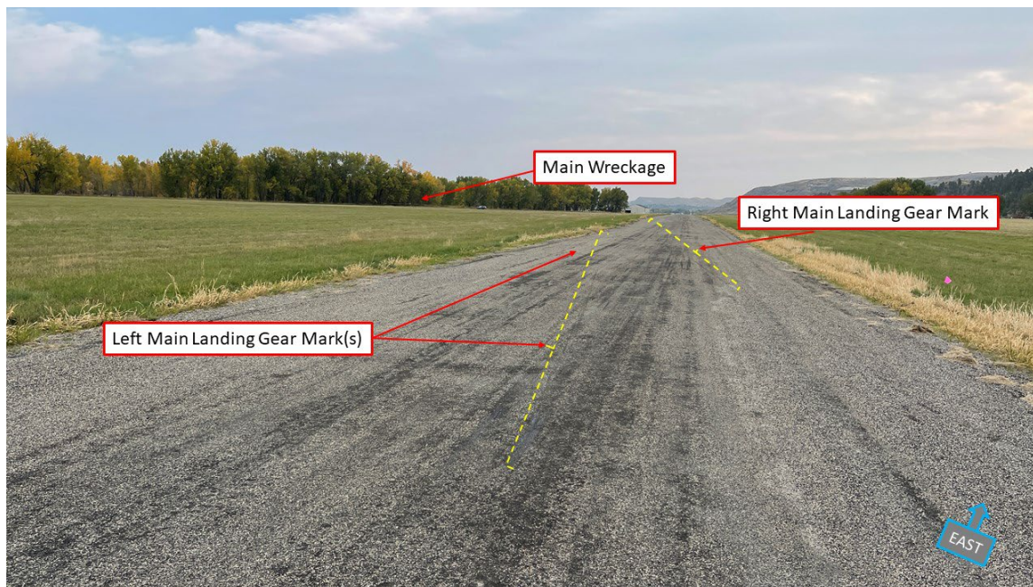
Figure 1: Runway marks with annotations.
