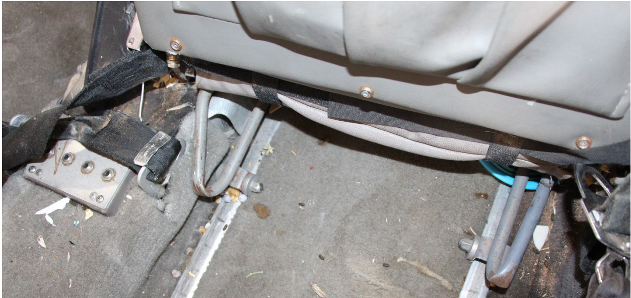
Photograph 4: Seat no. 2 aft frame tubes and seat tracks
