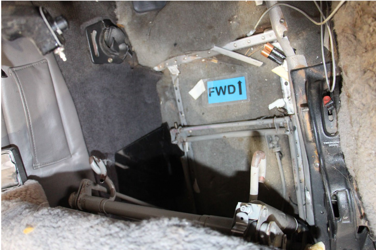
Photograph 3: Seat no. 1 forward tubes and seat tracks
