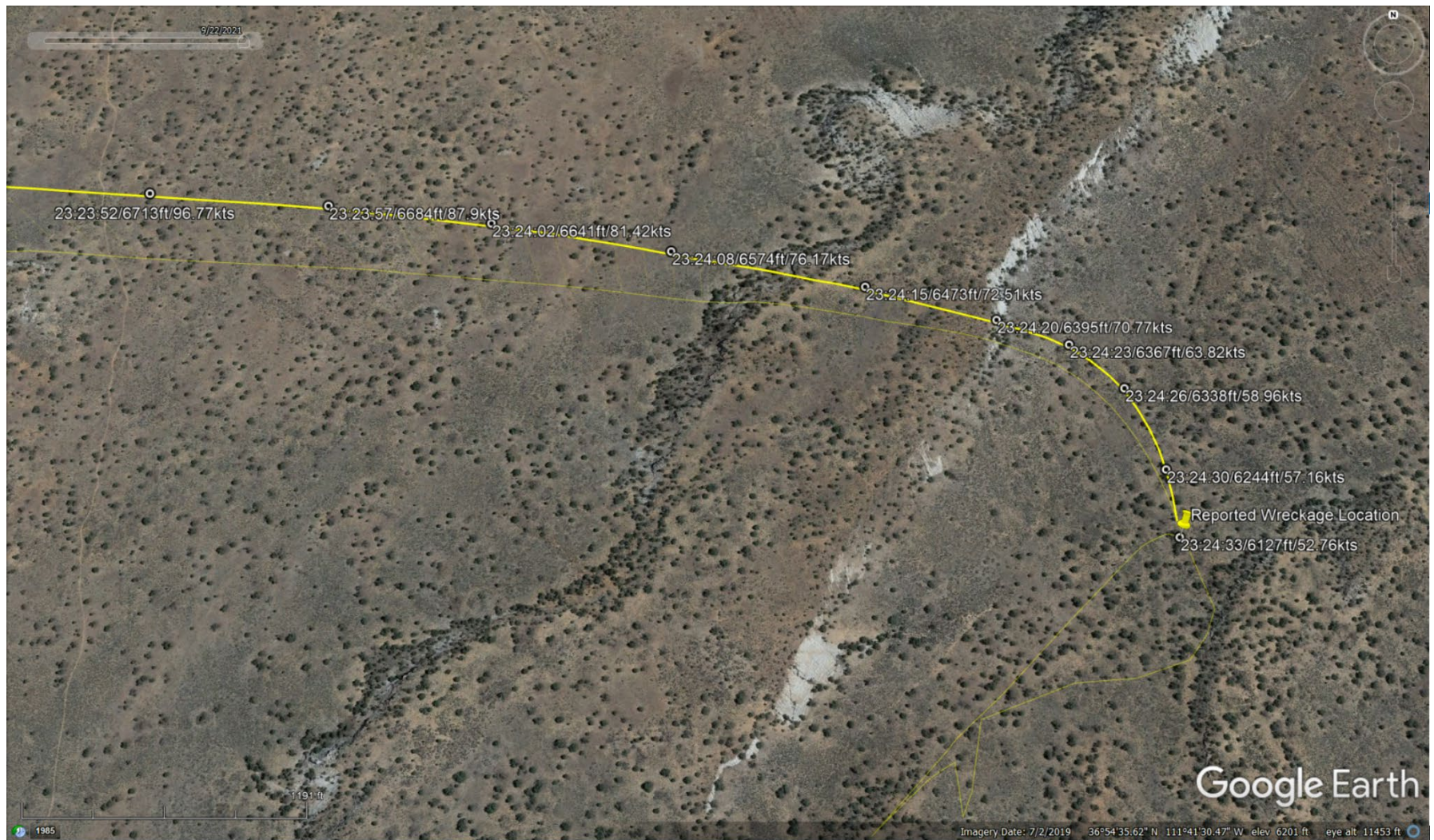
Figure 4. Google Earth overlay of the end of the event flight recorded on the Appareo Stratus 3.
