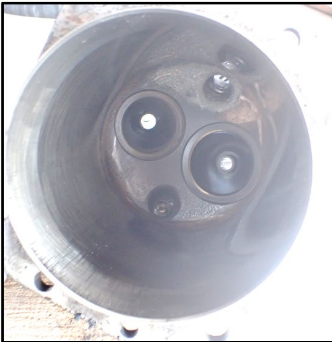
Figure 12: Cylinder No. 3 (Showing Cylinder Barrell and Piston Skirt Scuffs/Grooves)
