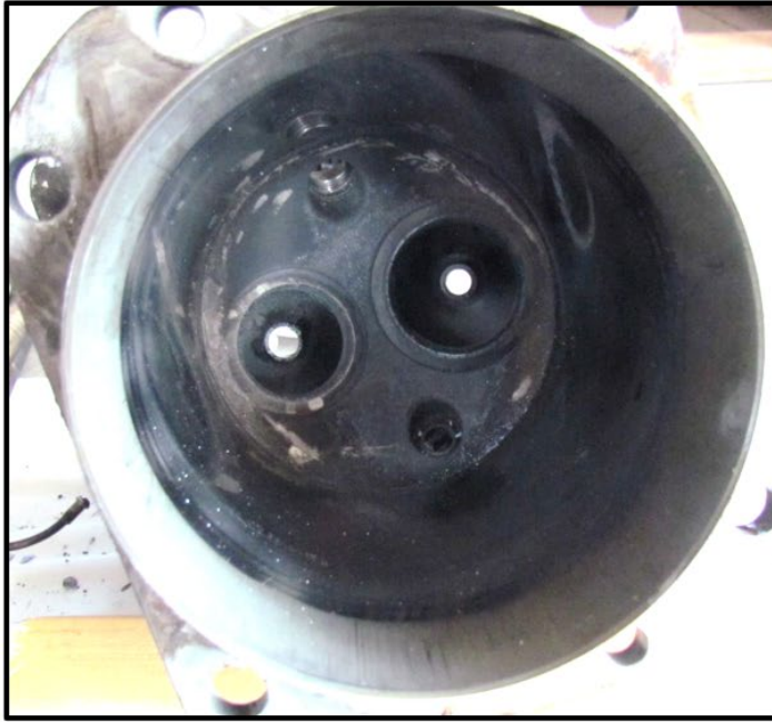
Figure 13: Cylinder No. 4 (Showing Cylinder Barrel and Piston Skirt Scuffs/Grooves)
