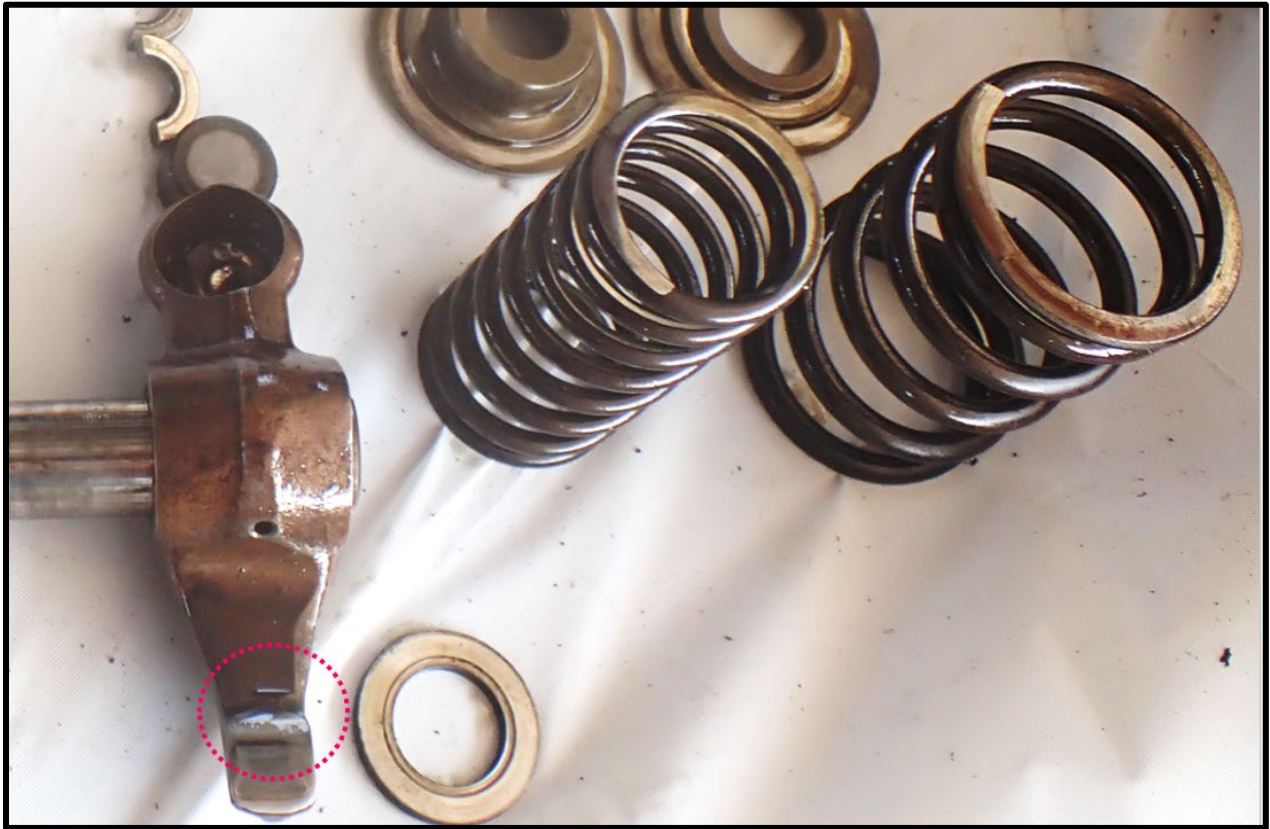
Figure 17: No. 4 Intake Rocker Arm and Valve Springs
