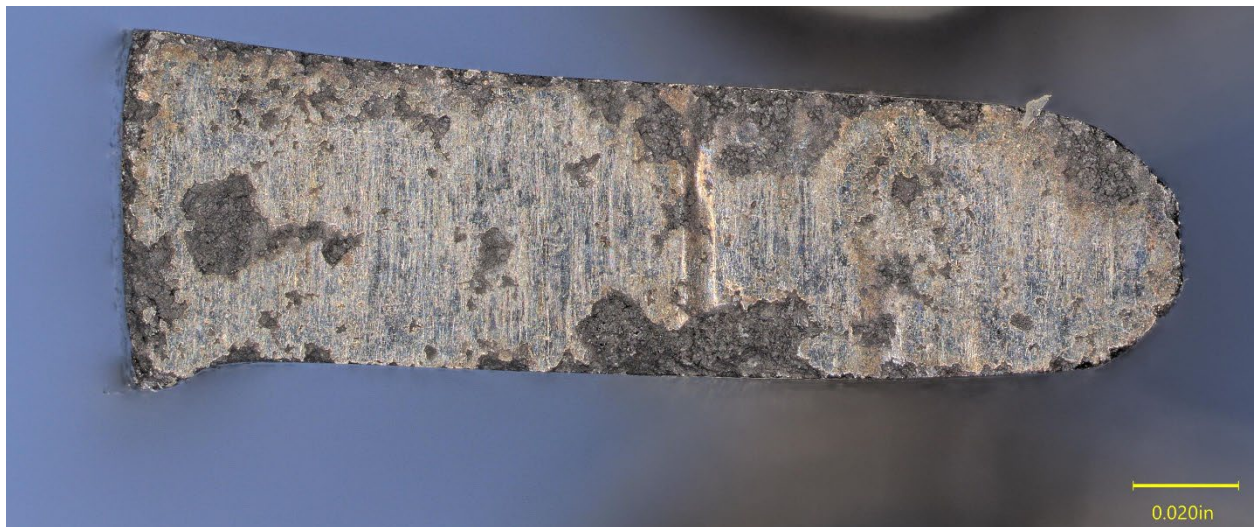
Figure 10. Surface 'A' from the ring fragment #1.
