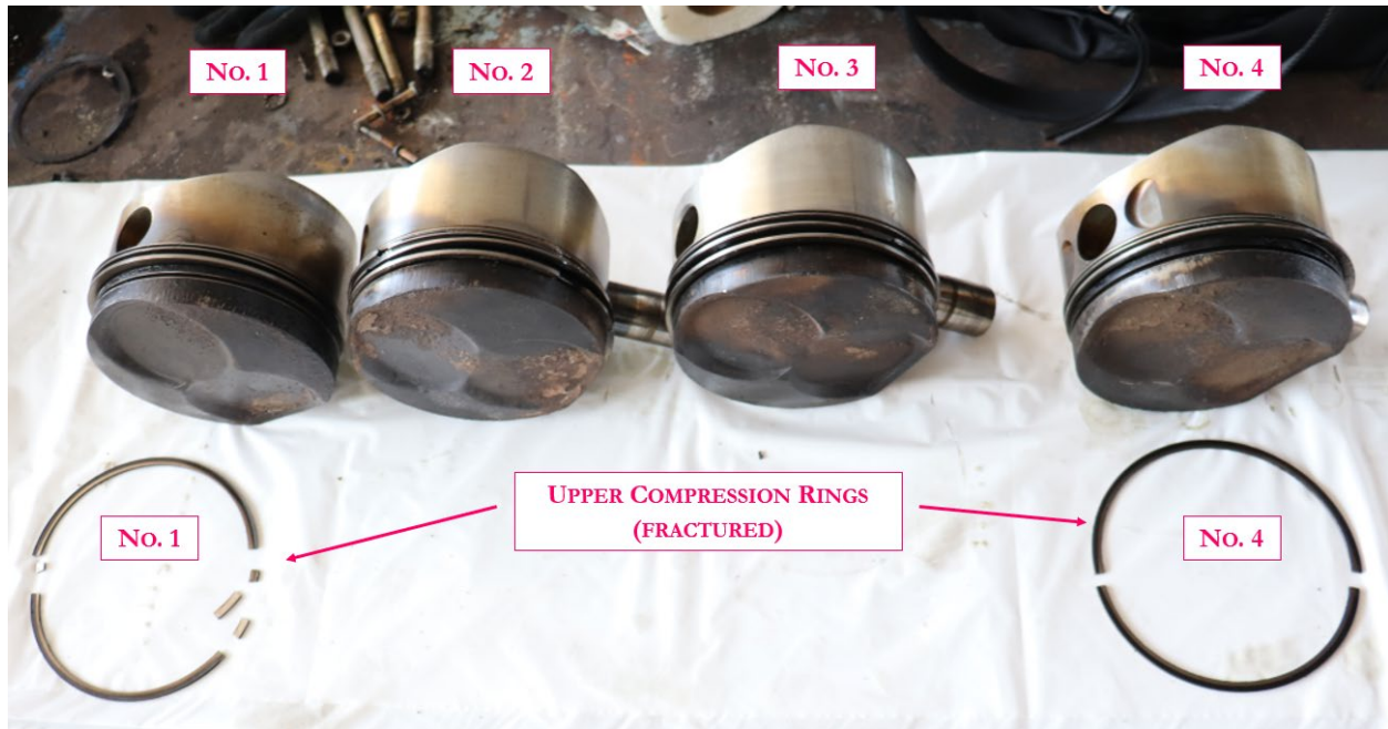
Figure 1. Images of the pistons and fracture rings from the engine teardown.
