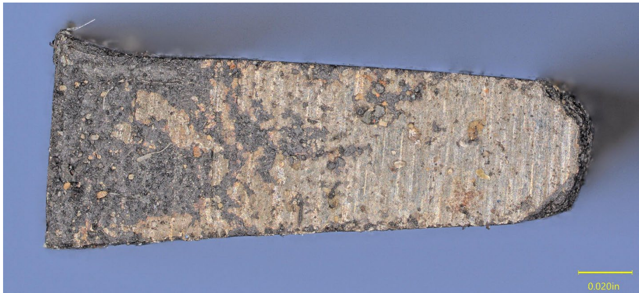
Figure 21. Surface 'B' from the shorter #4 ring remnant.
