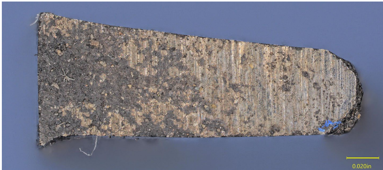
Figure 19. Surface 'B' from the longer #4 ring remnant.
