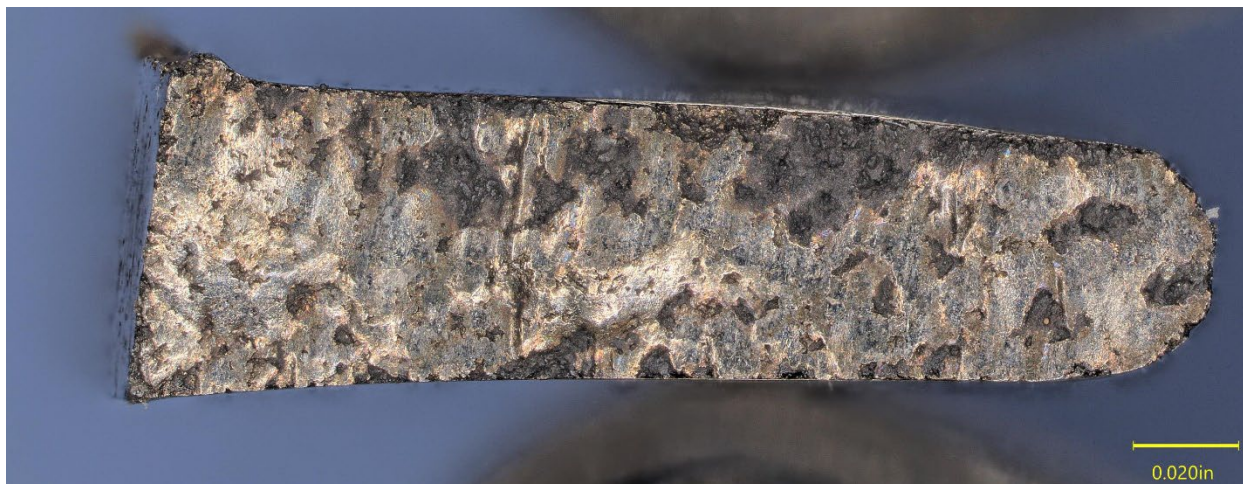
Figure 17. Surface 'B' from the ring fragment #4.
