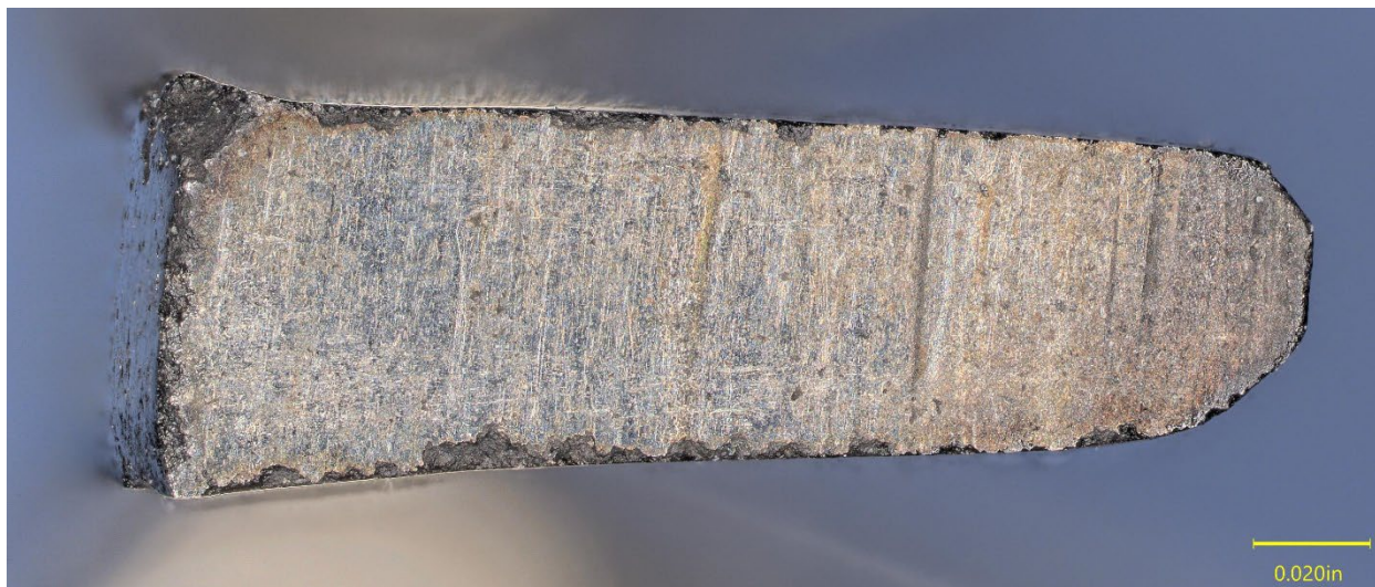
Figure 11. Surface 'B' from the ring fragment #1.
