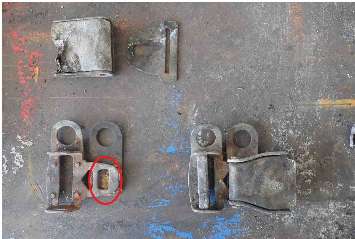
Figure 2 – Seat belt buckles, circle indicates shiny unburnt surface of tongue
