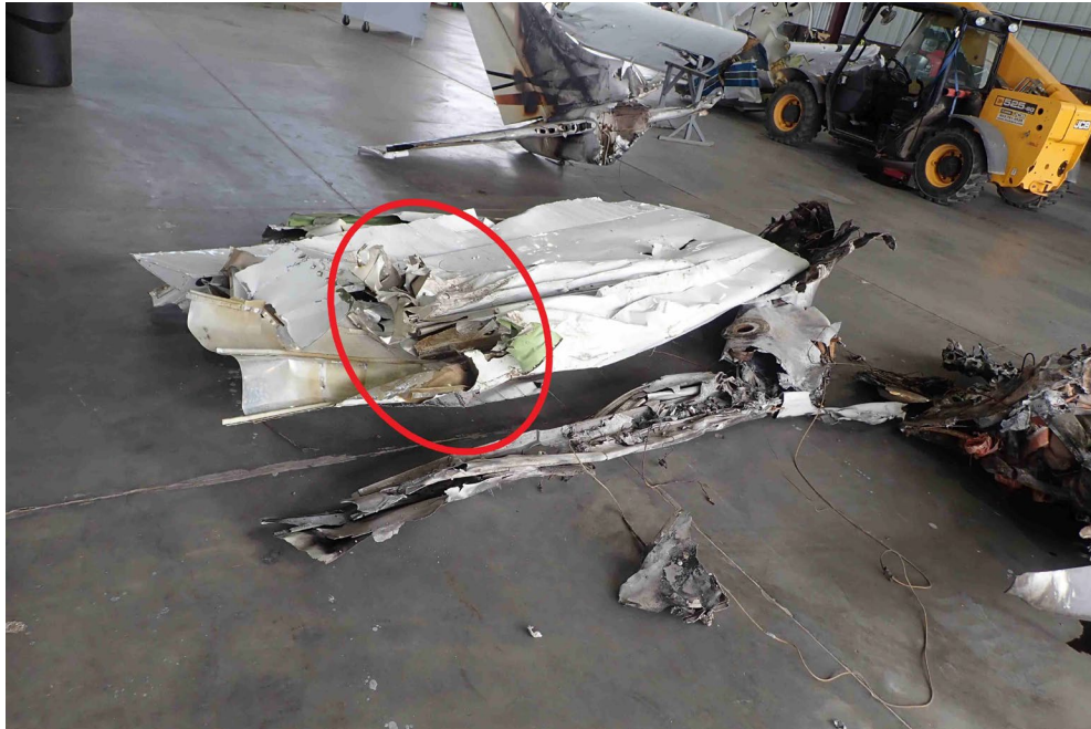
Figure 5 – Tree damage to right wing leading edge and underside
