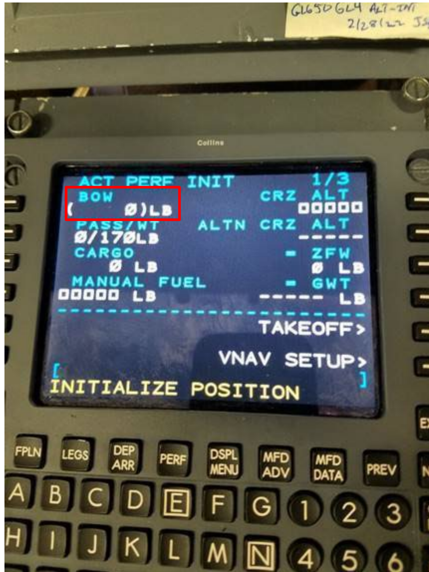
Figure 2 - After clearing the FMC the BOW is cleared as shown. BOW value is boxed in red. (Photograph courtesy of Collins Aerospace)
