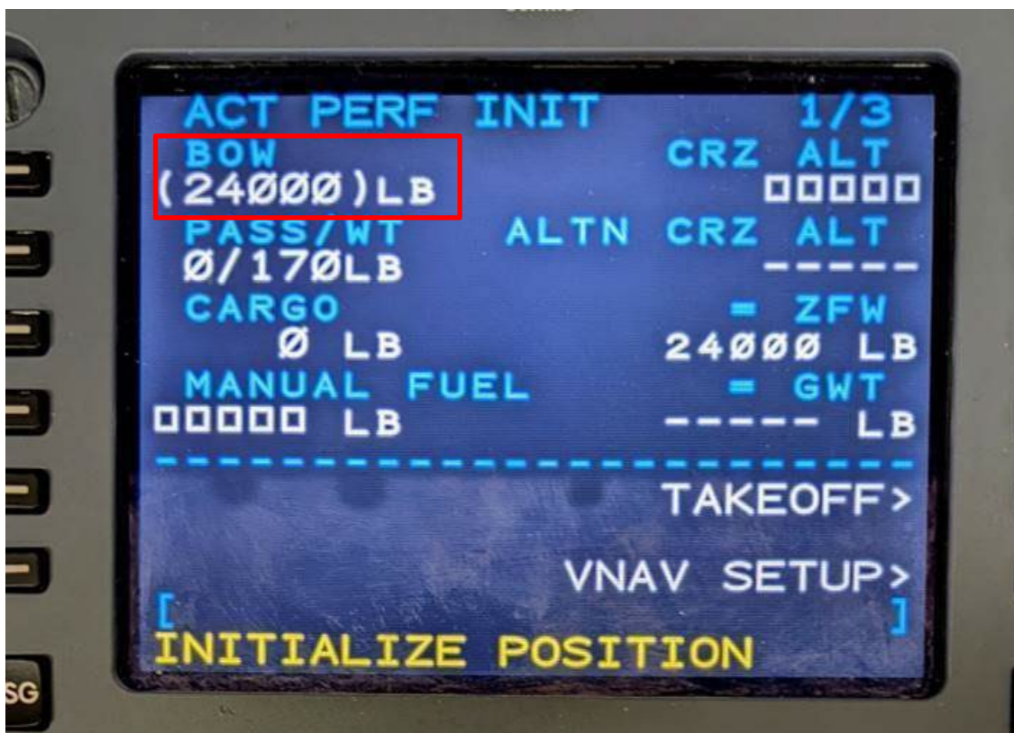
Figure 3 - After re-installing the performance databases, the default BOW is 24,000 pounds, as shown in red box. (Photograph courtesy of Collins Aerospace)
