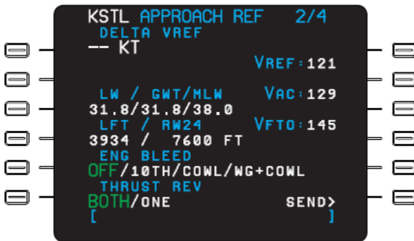
Figure 24: FMS Control Display Unit (CDU) showing an example of APPROACH REF page 2/4. 120
