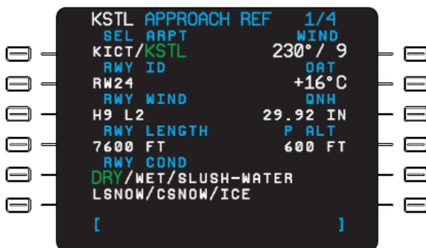
Figure 23: FMS Control Display Unit (CDU) showing an example of APPROACH REF page 1/4. 119
