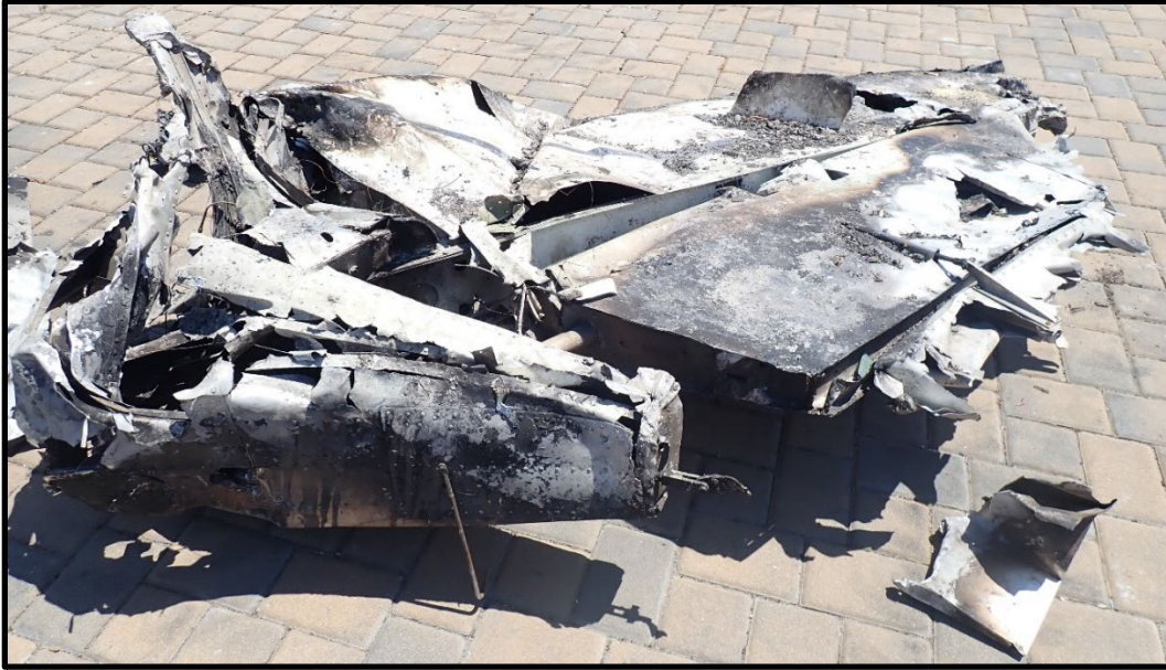
Figure 10: View of vertical stabilizer and rudder (photo courtesy of the NTSB)
