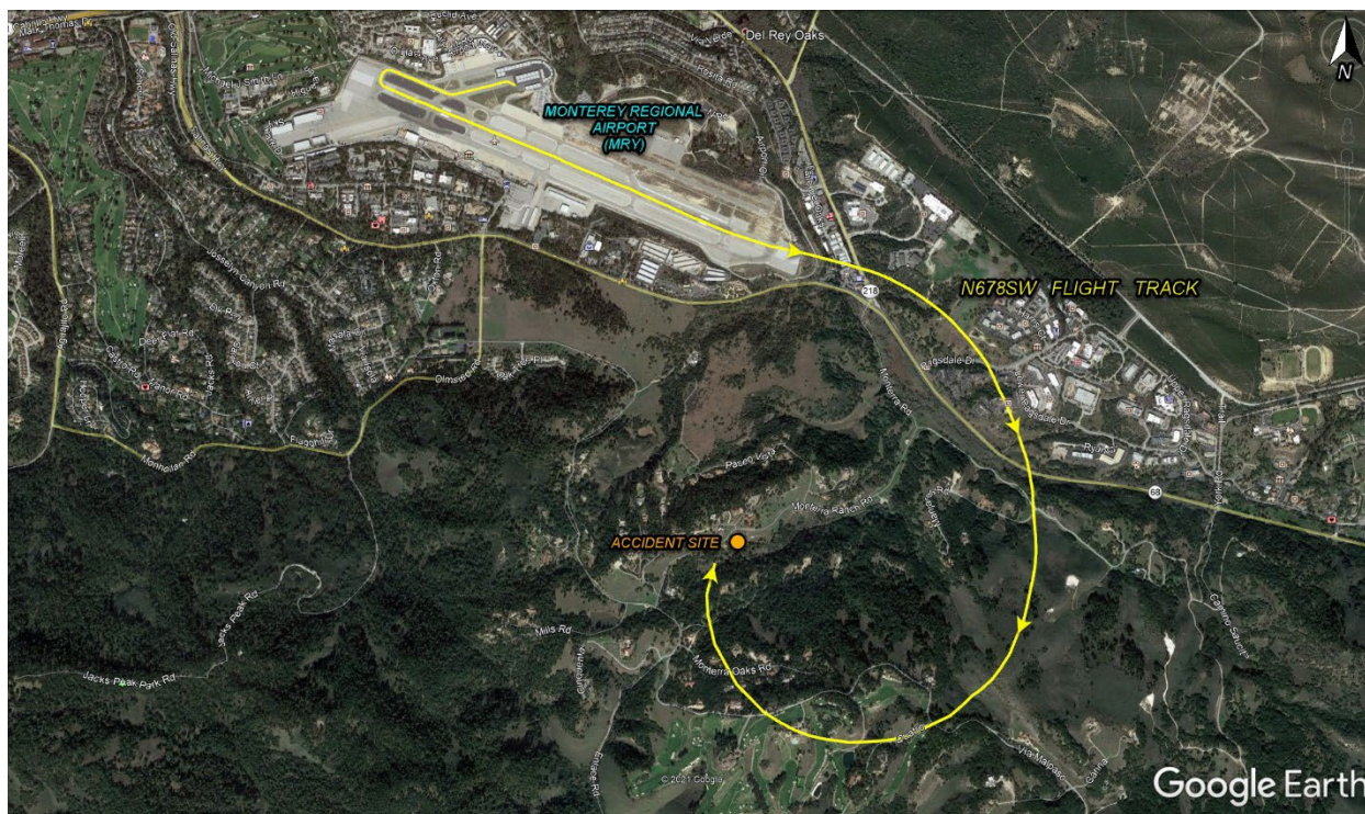
Figure 1. Overhead view of accident flight track overlaid onto satellite imagery.
