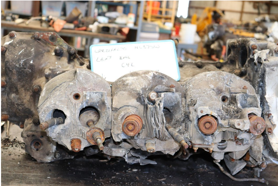
Figure 11: View of left engine cylinders 2, 4, and 6. (Photo courtesy of the NTSB)
