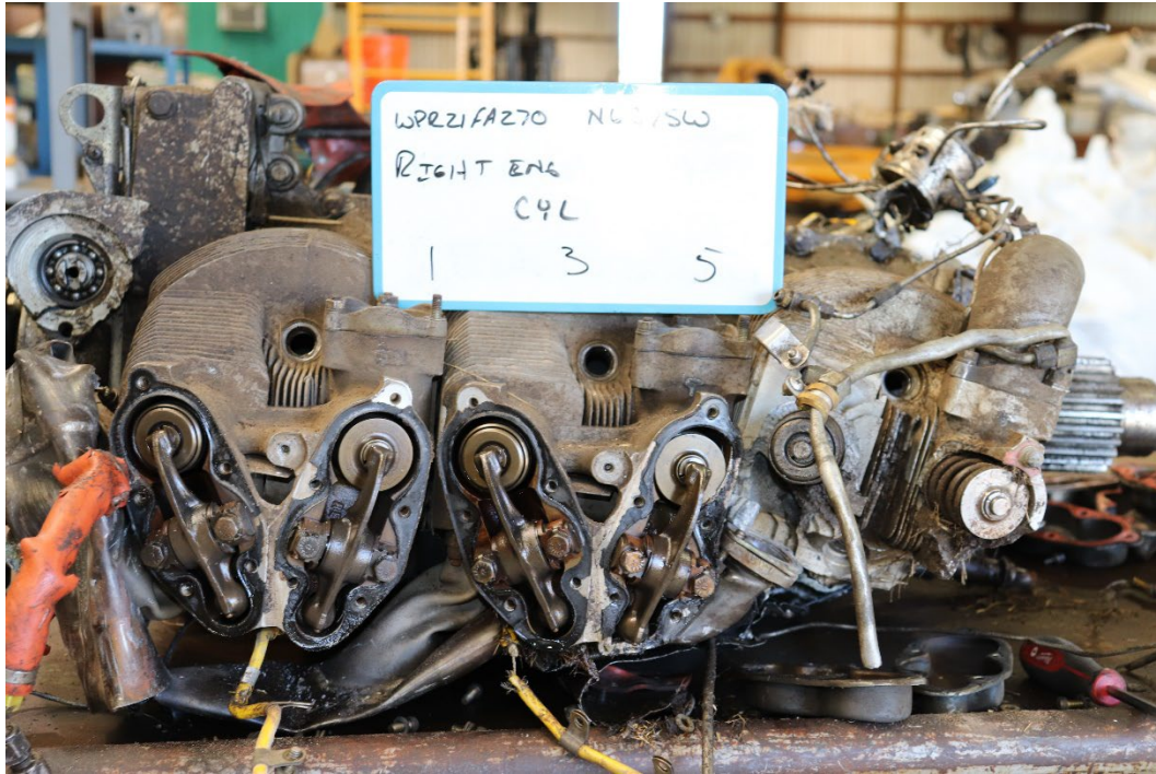
Figure 22: View of right engine cylinders 1, 3, and 5. (Photo courtesy of the NTSB)
