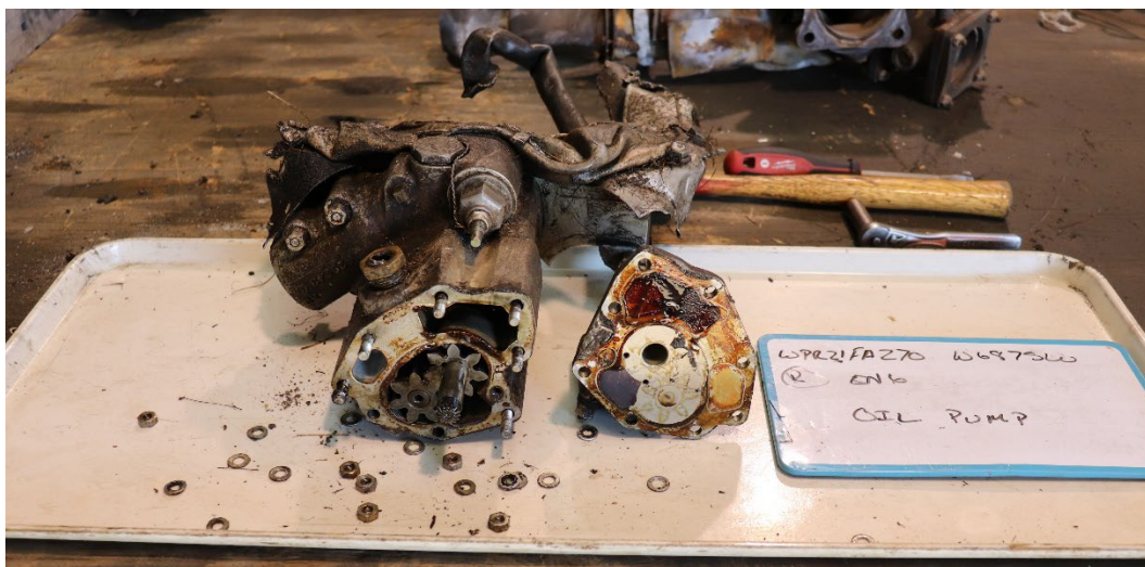
Figure 27: View of right engine oil pump. (Photo courtesy of the NTSB)
