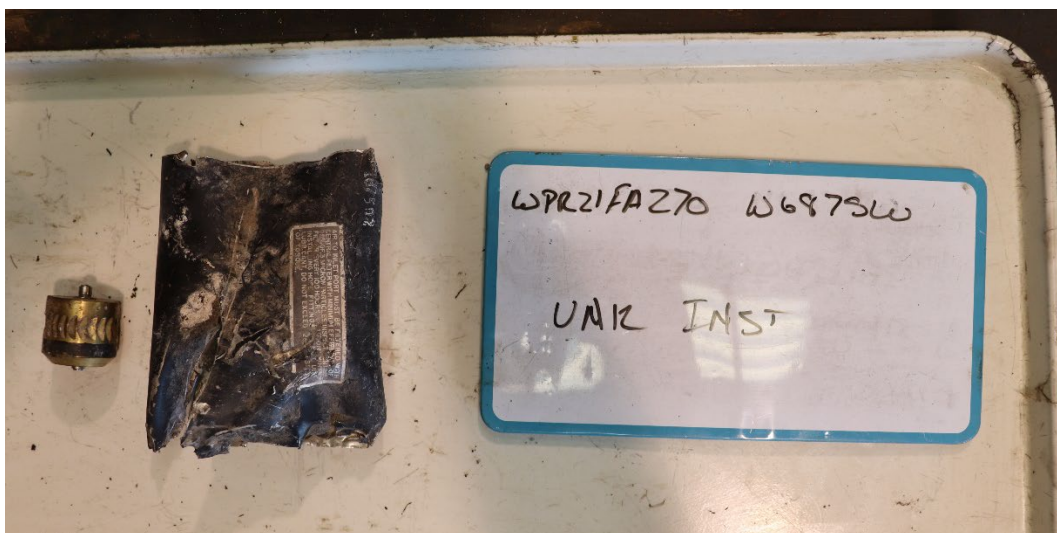
Figure 3: View of unknown instrument with impact and thermal damage. (Photo courtesy of the NTSB)
