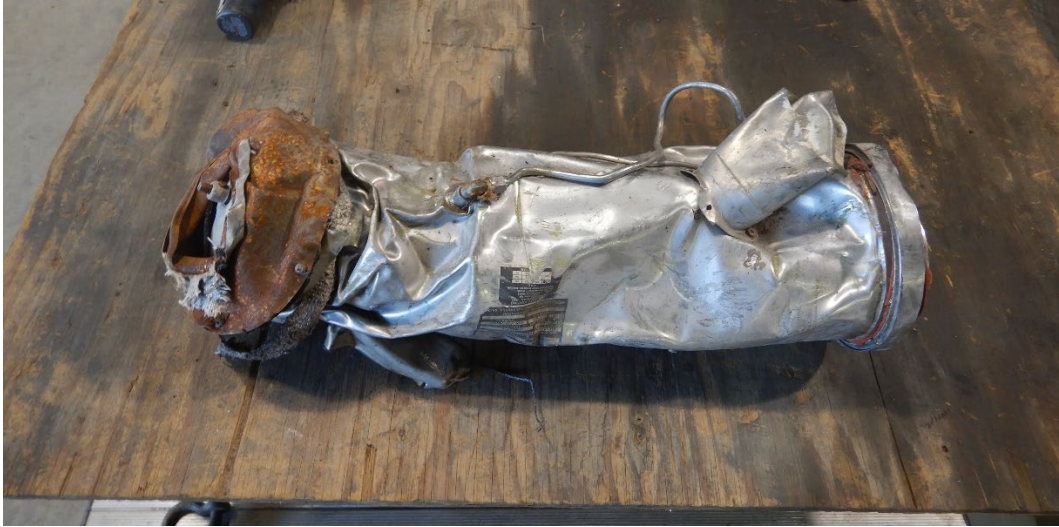
Figure 9: View of airplane heater assembly with impact and thermal damage. (Photo courtesy of Textron Aviation)
