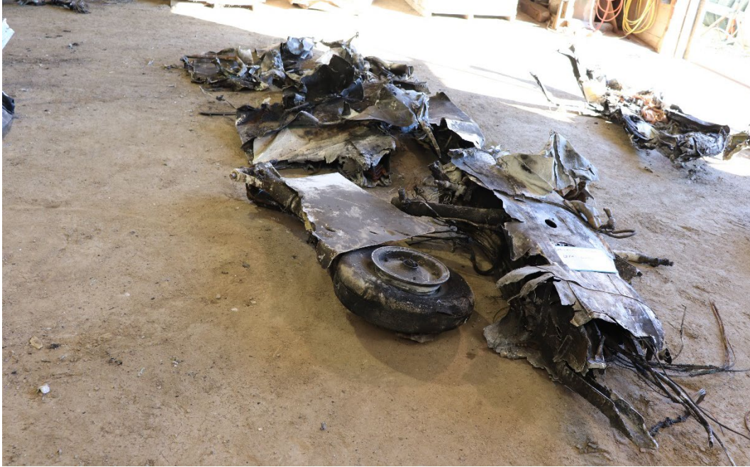
Figure 6: View of left wing with impact and thermal damage. (Photo courtesy of the NTSB)
