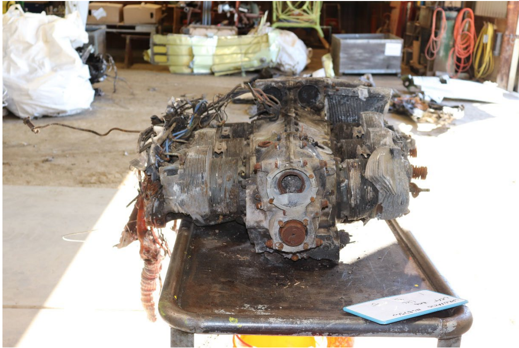
Figure 10: Front view of left engine with impact and thermal damage. (Photo courtesy of the NTSB)
