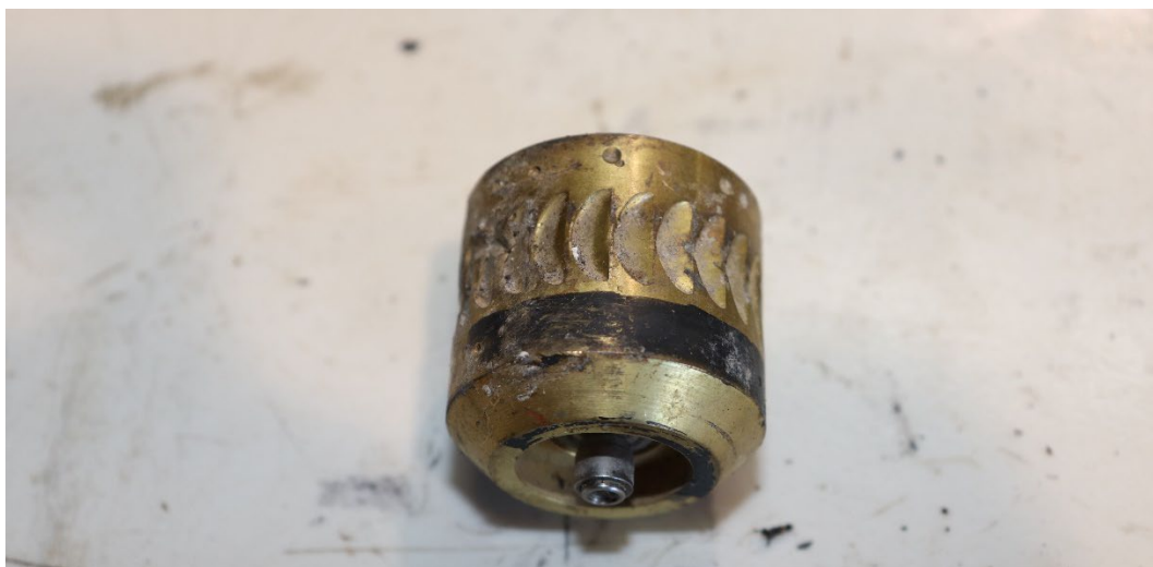
Figure 4: View of unknown instrument gyro gimble with rotational scoring and impact damage. (Photo courtesy of the NTSB)
