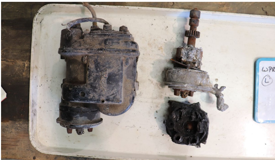
Figure 15: View of left engine magnetos. (Photo courtesy of the NTSB)
