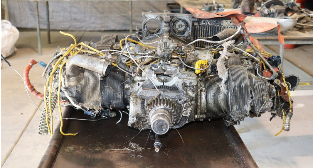
Figure 20: Front view of right engine with impact damage. (Photo courtesy of the NTSB)
