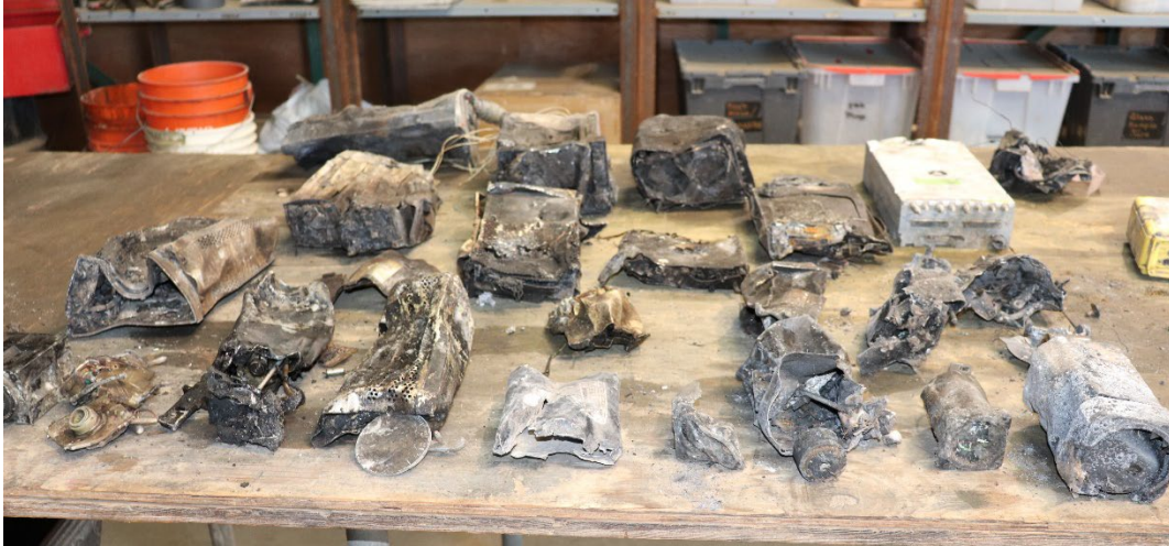
Figure 2: View of various airplane instruments with impact and thermal damage. (Photo courtesy of the NTSB)
