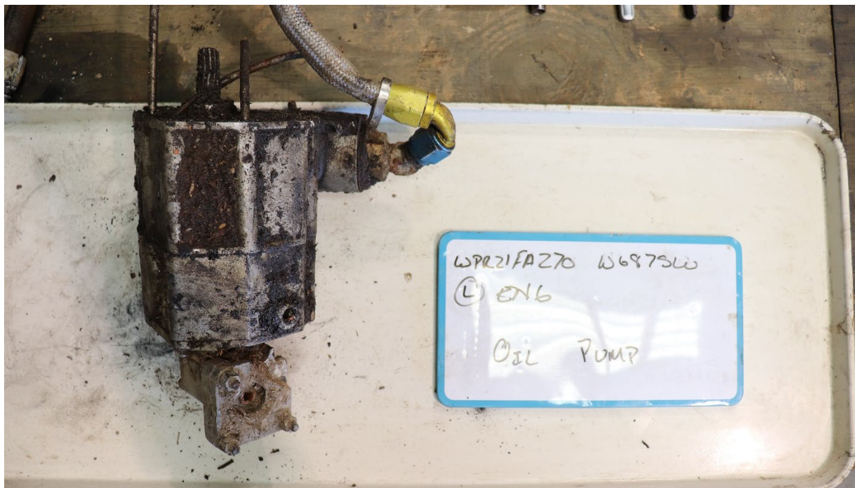
Figure 19: View of left engine oil pump. (Photo courtesy of the NTSB)
