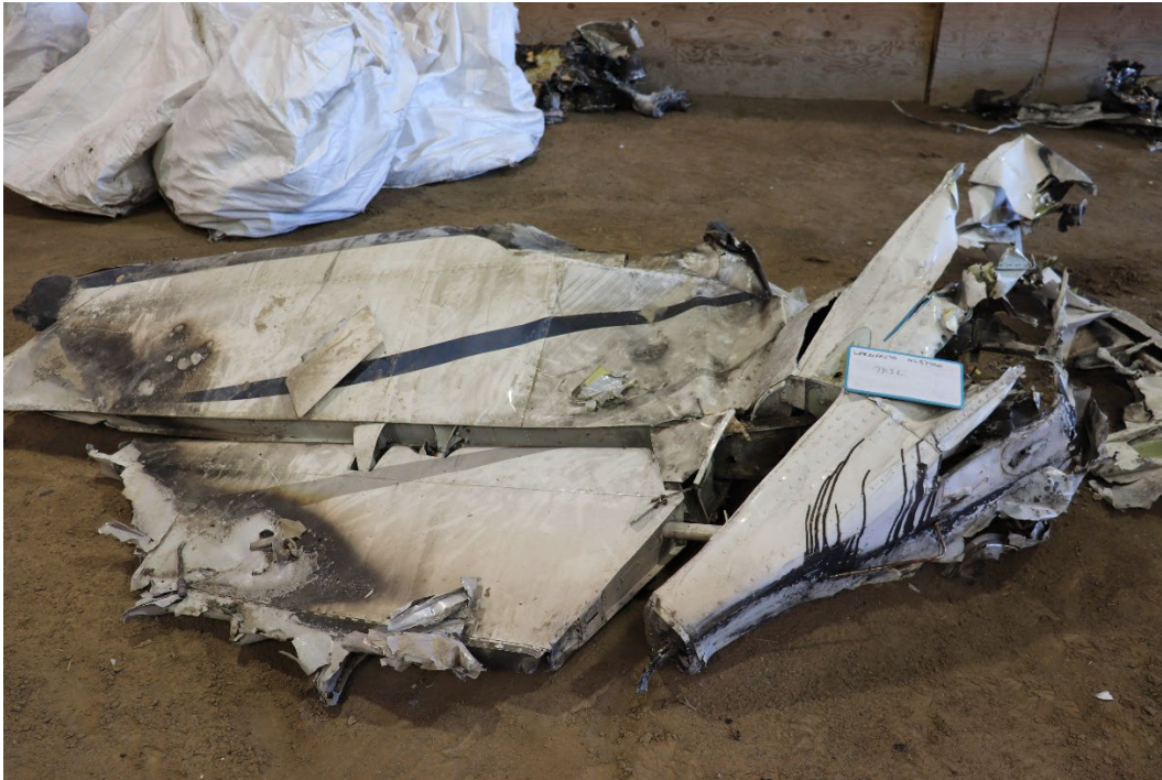
Figure 8: View of empennage with impact and thermal damage. (Photo courtesy of the NTSB)
