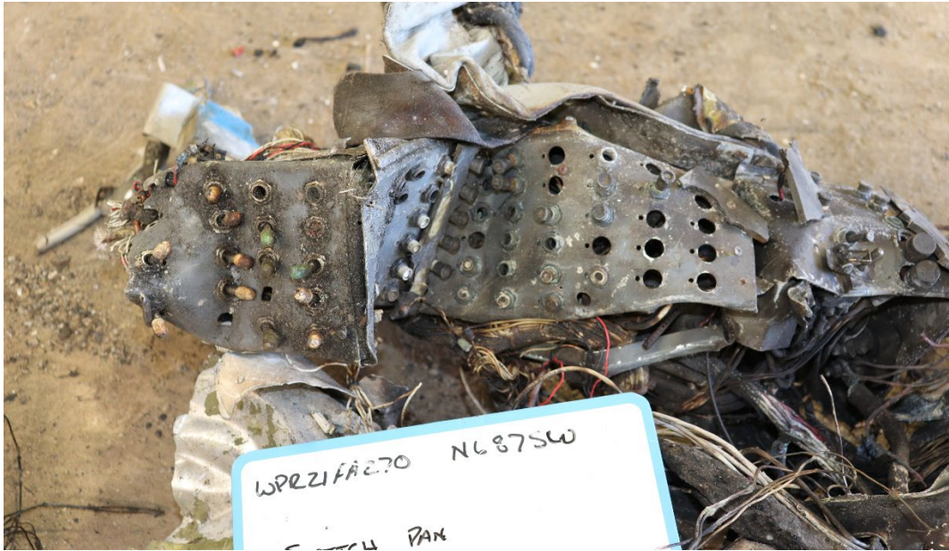
Figure 5: View of airplane cockpit switch/circuit breaker panel with impact and thermal damage. (Photo courtesy of the NTSB)
