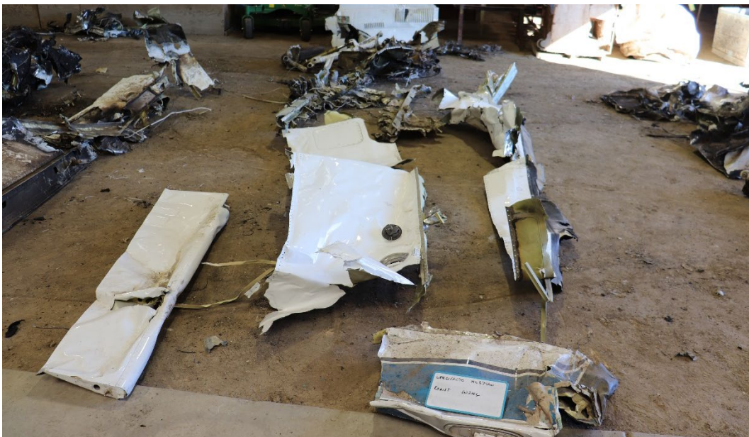
Figure 7: View of right wing with impact and thermal damage. (Photo courtesy of the NTSB)
