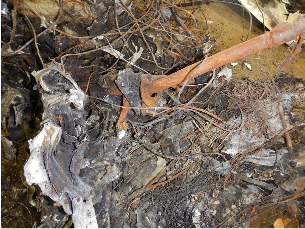
Figure 1: View of airplane cockpit area with impact and thermal damage. (Photo courtesy of Textron Aviation)
