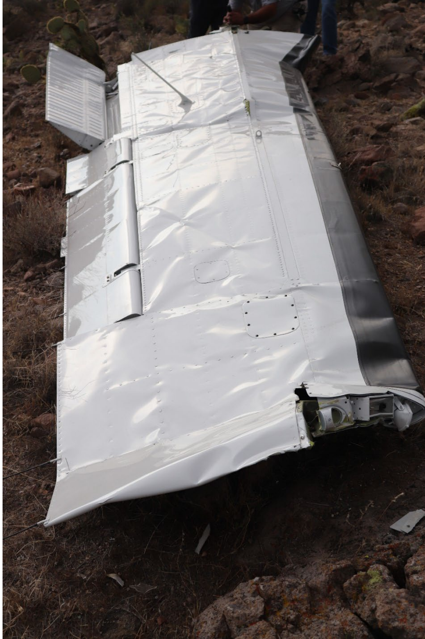
Figure 6: Left wing as located at the accident site viewed from the outboard section.
