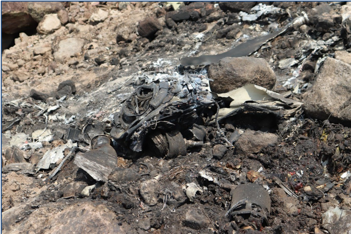
Figure 2. Engine A and 3 blades within the main wreckage site.
