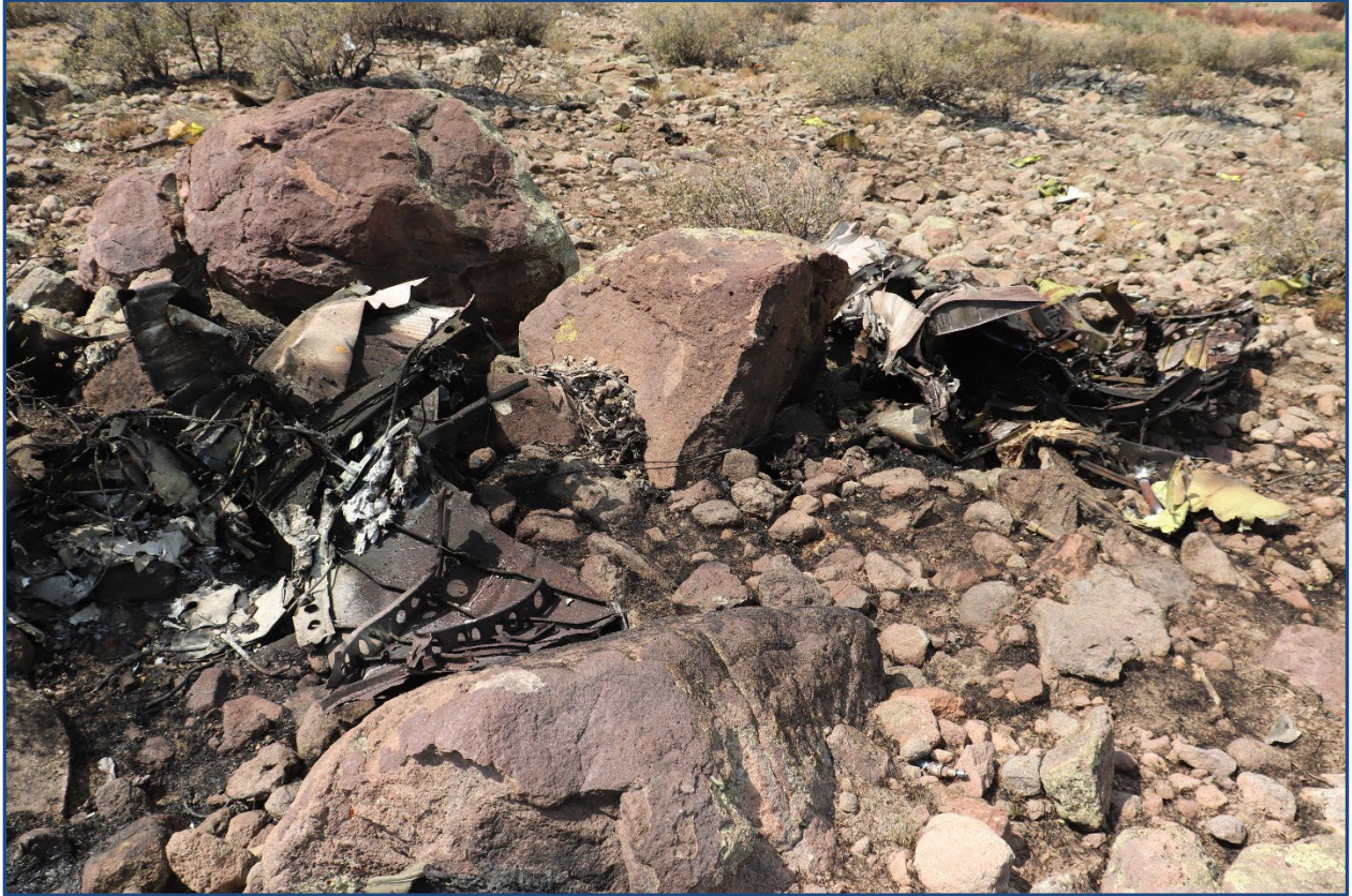
Figure 4: Two sections of the right wing.
