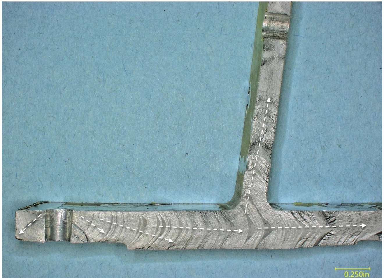
Figure 1 – Fracture surface of the fatigue crack on the lower wing spar cap, after disassembly, sectioning, and cleaning. The white dashed arrows denote the general crack propagation direction from the fastener hole.
