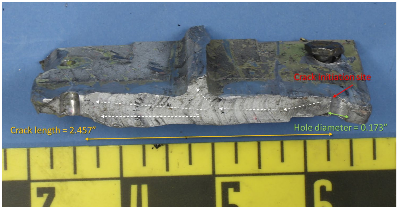
Figure 9 – View of the fracture surface of the inboard lower spar cap fracture surface, after sectioning.
