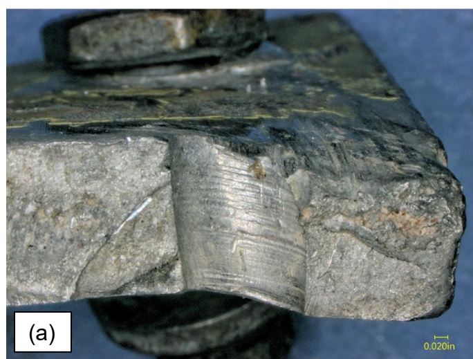
Figure 14 – View of the fastener hole in the inboard lower spar cap (a) overall and (b) closer, showing circumferential gouges on the surface.
