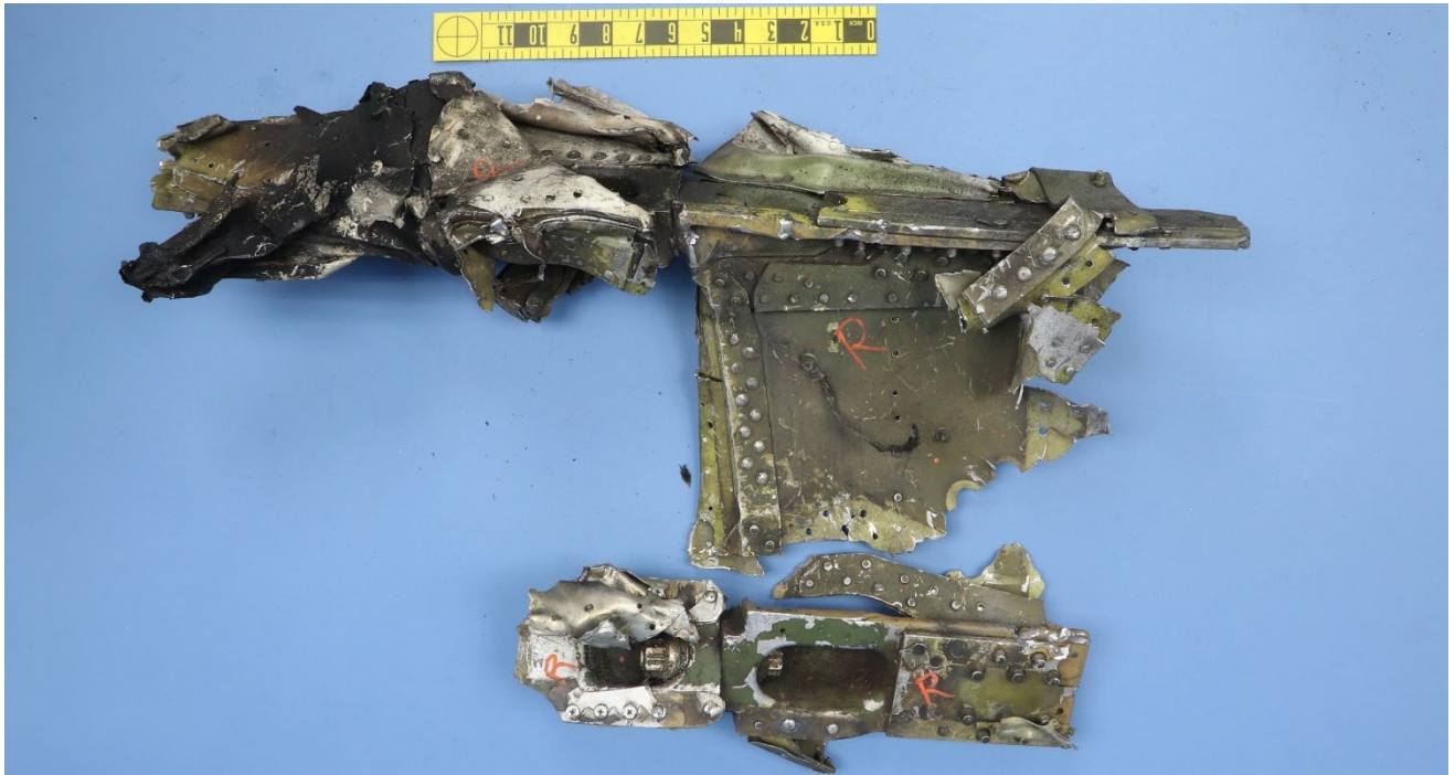
Figure 31 – Reconstruction of right wing spar fragments.
