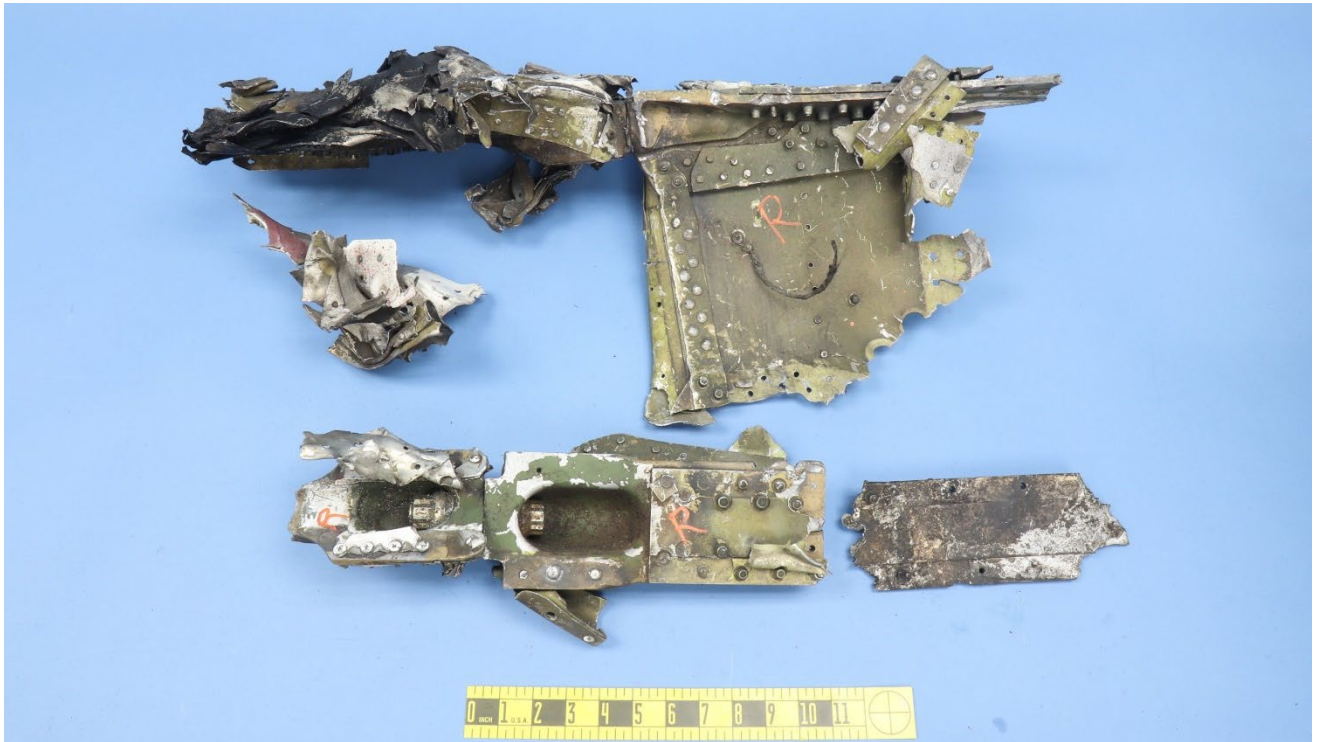
Figure 29 – View of the wing spar components from the right side.
