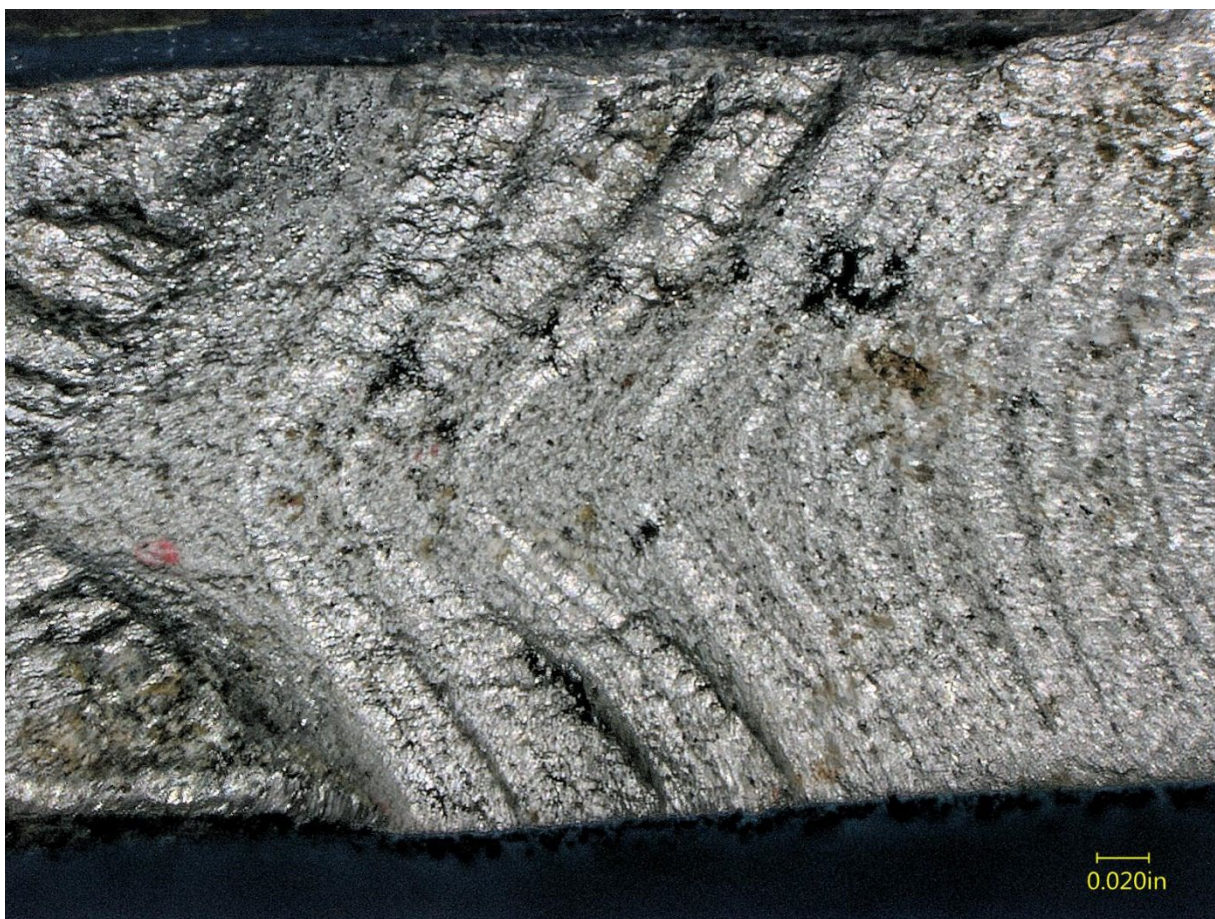
Figure 13 – Fracture surface of the inboard lower spar cap away from fastener hole
