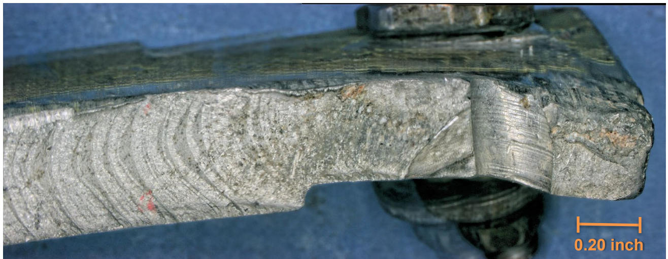
Figure 10 – Close view of the inboard lower spar cap fracture surface near the fastener hole initiation site.
