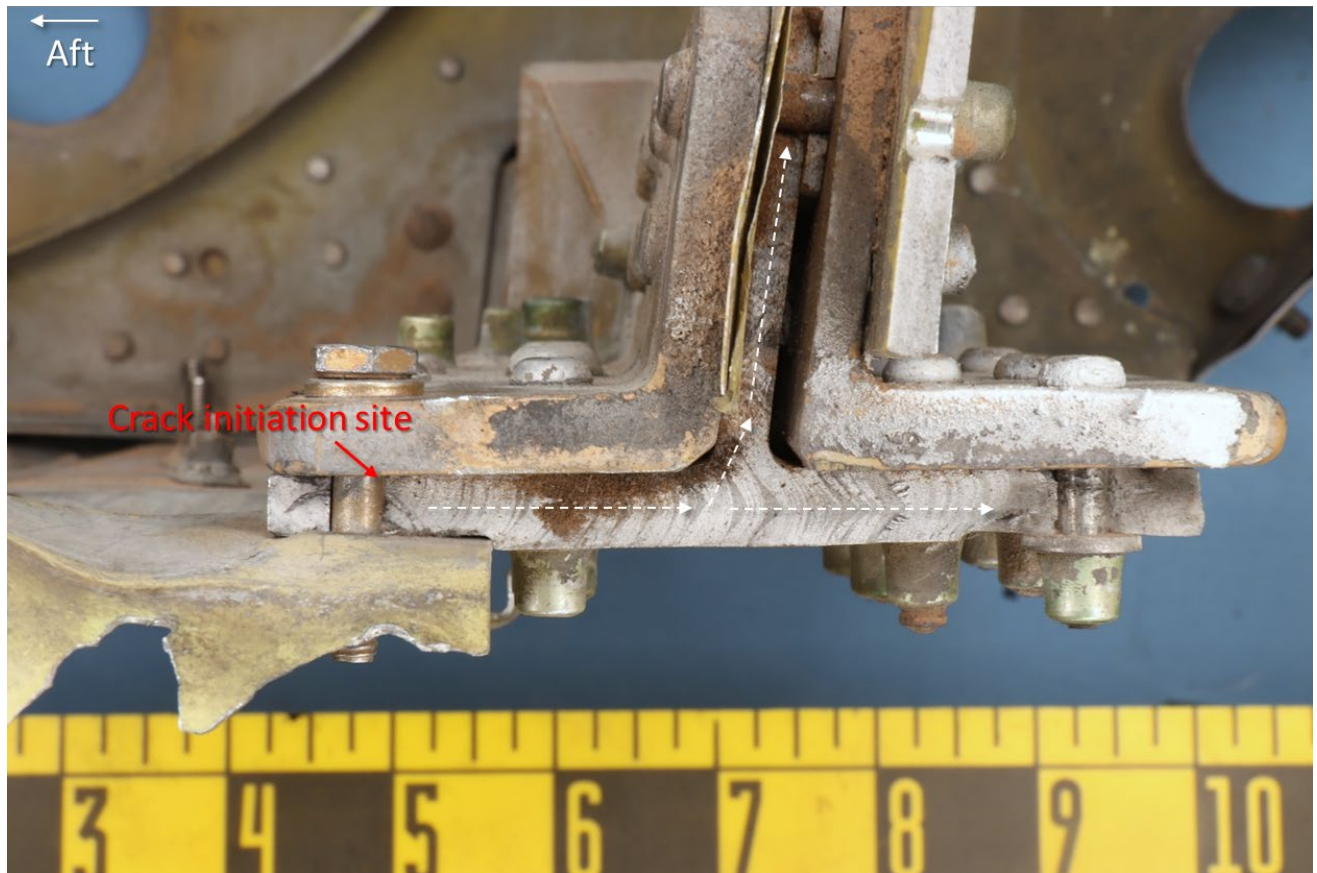
Figure 3 – Fracture surface of the lower outboard spar cap remnant, as received, annotated to show the general crack initiation site and direction of crack propagation.
