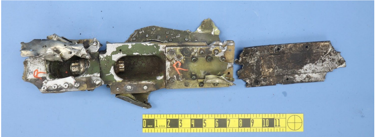
Figure 30 – Reconstruction of the lower wing spar cap and wing fittings.
