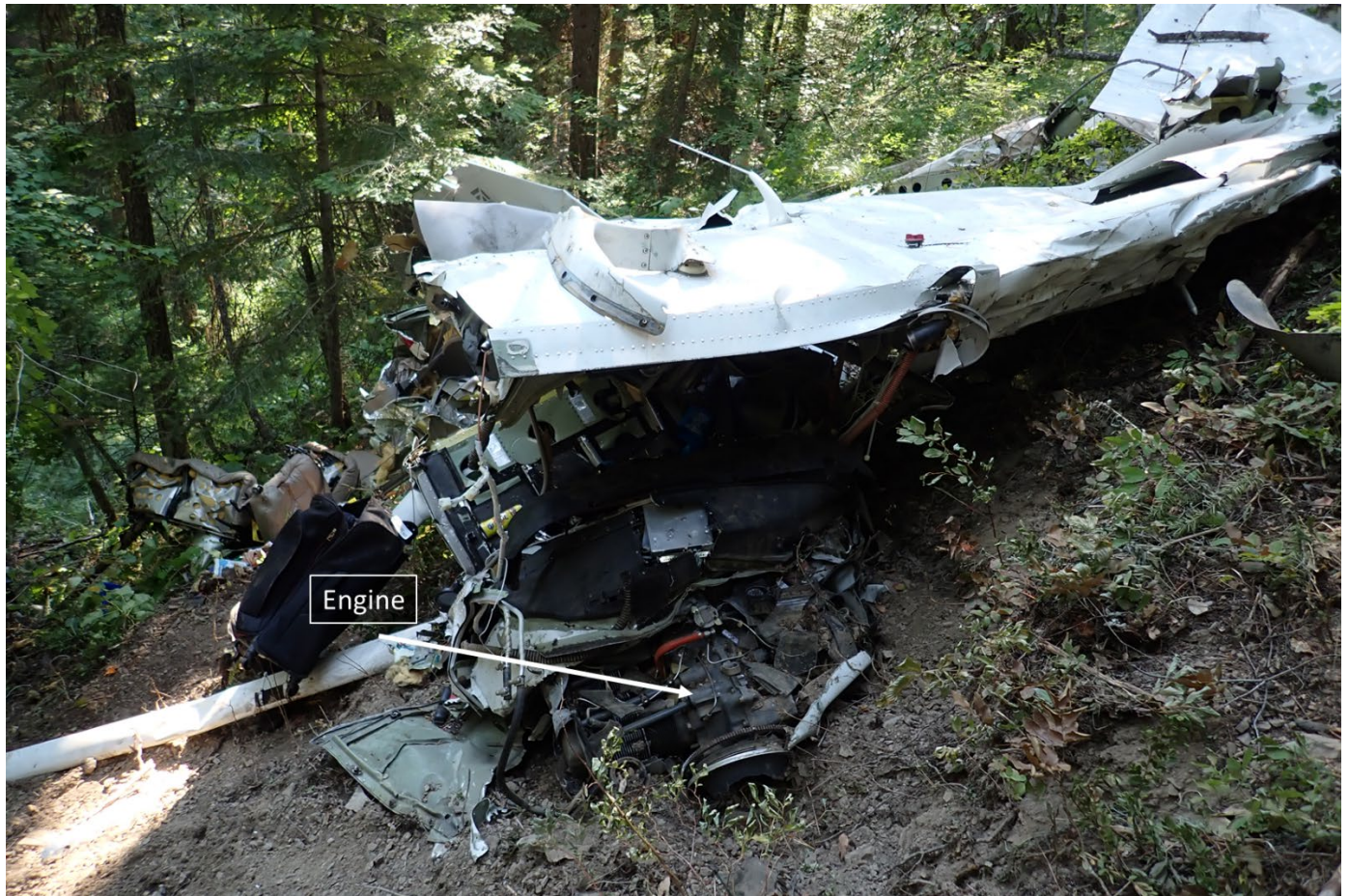
Figure 6. Engine and cabin roof.
