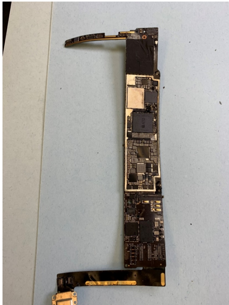
Figure 2: Damaged iPad mini 5 motherboard.
