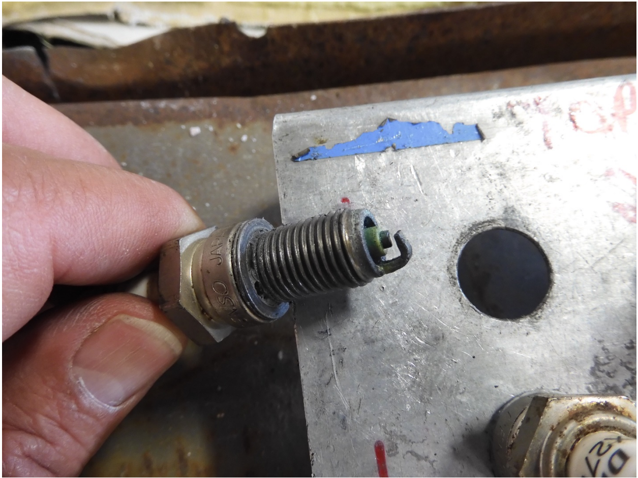
Figure 21. Example of one spark plug electrode, showing gap and wear.
