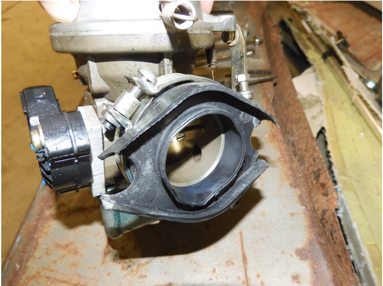
Figure 19. 2, 4 Carburetor showing the torn rubber flange assembly.
