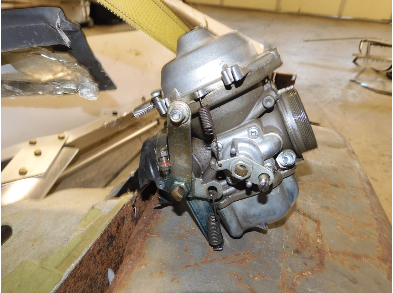
Figure 18. 2, 4 Carburetor, showing external fuel staining.
