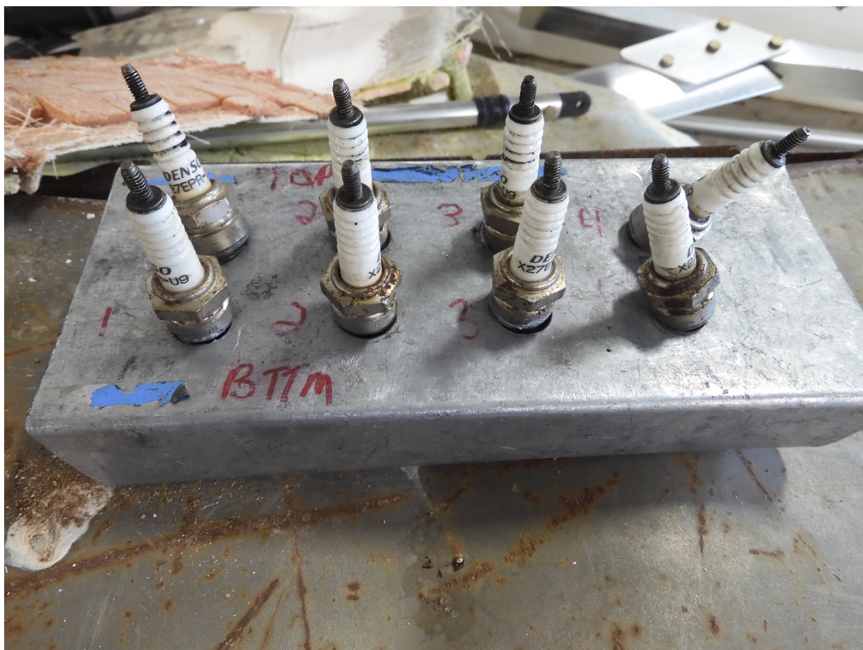
Figure 20. Spark plugs removed from the accident engine.
