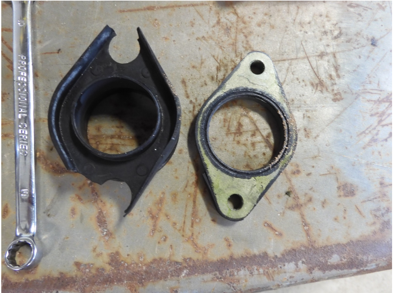
Figure 16. Torn rubber flange assembly for the 1, 3 carburetor.
