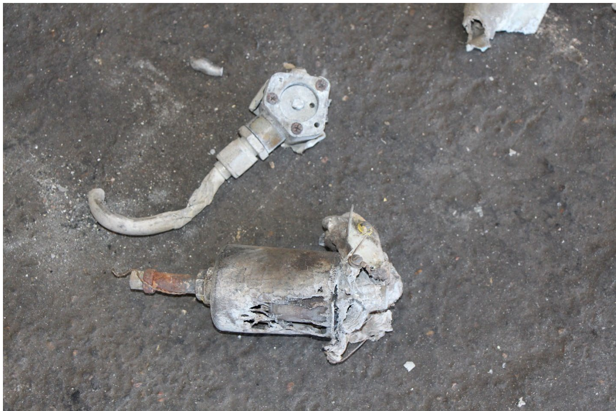
Photograph 2: Gascolator and Fuel Selector
